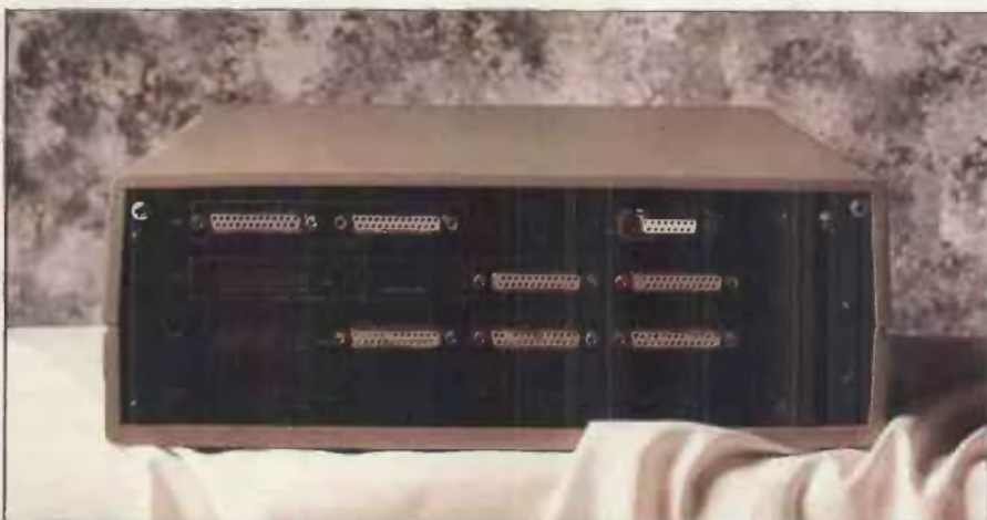
Seven standard DB25 connectors serve the Sprite's serial connectors
