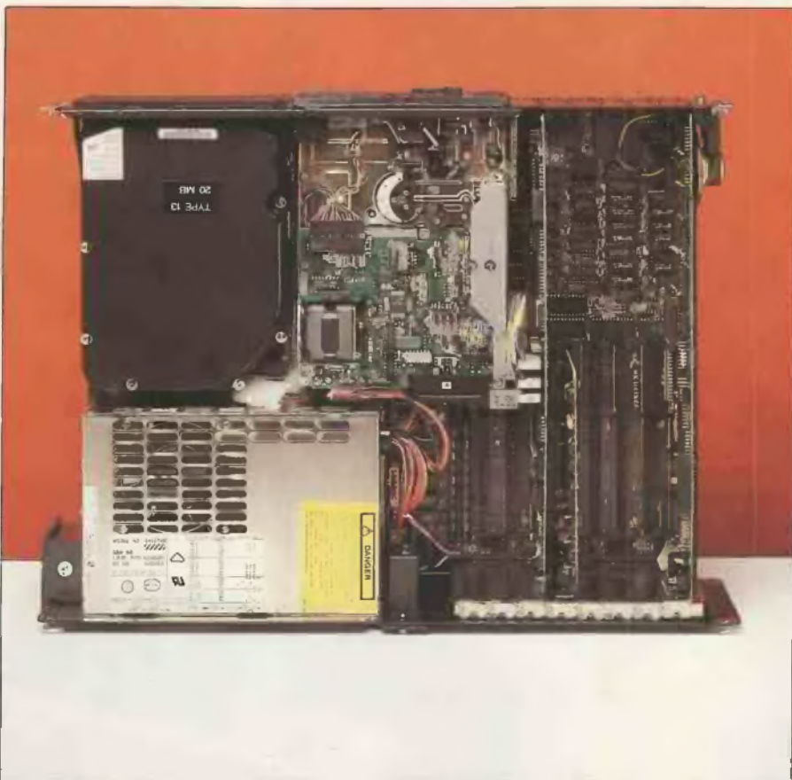
The XT 286 contains large amounts of TTL logic chips — there are no ULAs
