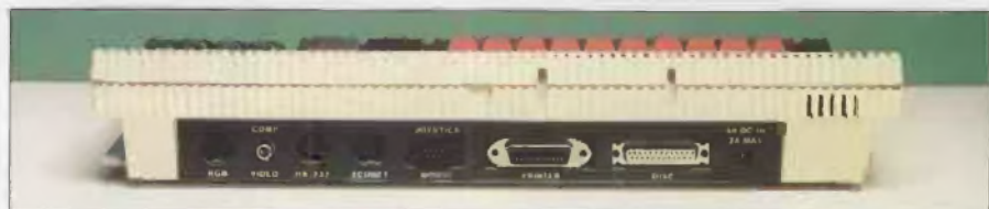
The user port on the old BBC machines has been re-cast on the Baby Beeb as a 9-pin interface for a joystick or mouse
