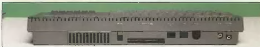
The +2's video port produces composite PAL and RGB signals, but several add-ons won't fit unless you use an extension cable
