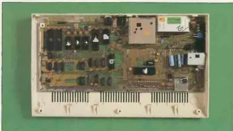
In electrical terms, the 64C is almost identical to the 64; the only obvious difference is the use of two high-capacity RAM chips for the 64k memory
