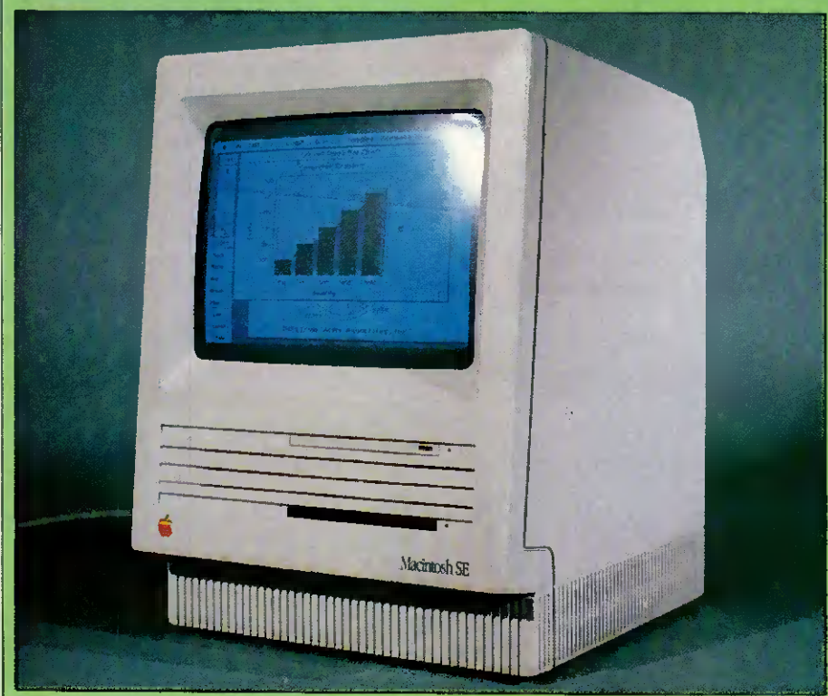
Externally the Mac SE is similar to the Mac Plus, but the drive slots are now stacked on top of one another rather than side by side (although the upper one here is blanked off). Inside is another story . . .
