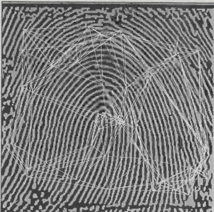
This thumb print was digitised and encoded by 16 transputers in 3.4 seconds. Forty-nine ridge endings and forks were found and linked to five neighbours
