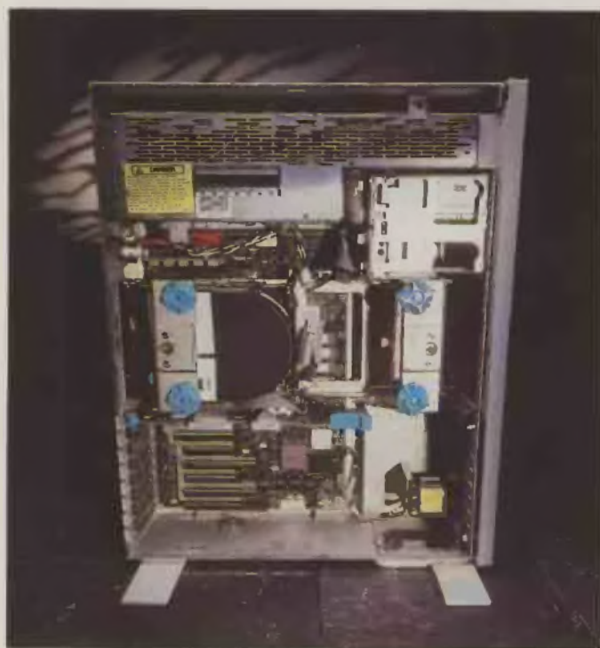
Inside the IBM PS/2 Model 80: the Micro Channel slots are visible below the hard disk and can take up to eight extension boards
