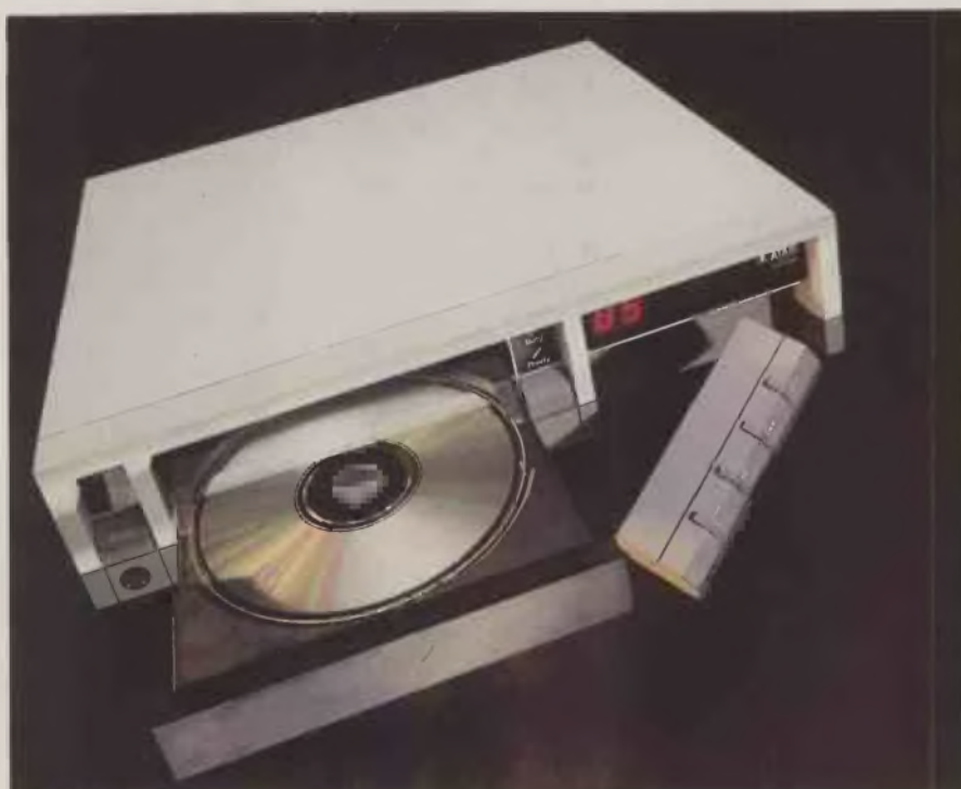
Inserting a compact disk is straightforward. Notice the removable remote control panel enabling the machine to be used as an ordinary CD player
