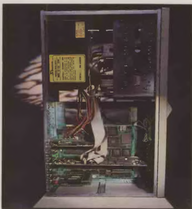
Surprisingly, Inter-Orient's CMC386 consists largely of empty space, with the computer itself being buried at the bottom of the tower
