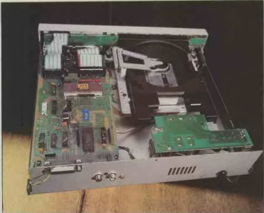
Looking at the Atari CD-001 from the rear: the player mechanism and power supply are visible to the right with the two PCBs to the left
