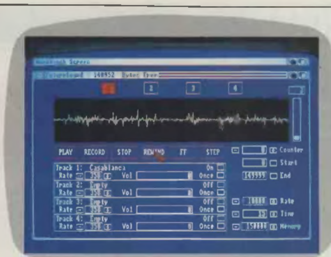
This Future Sound screen shows an immortal line from the film Casablanca as a Future Sound amplitude/time graph. Up to four tracks can be loaded in simultaneously
