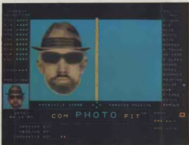
A screen from the ComPhotofit system, printed direct from the PC to polaroid film. The right-hand window originally held the image as selected by the witness from different component cards. It was then copied to the other window for rodential editing. The small picture shows a far view of the image
