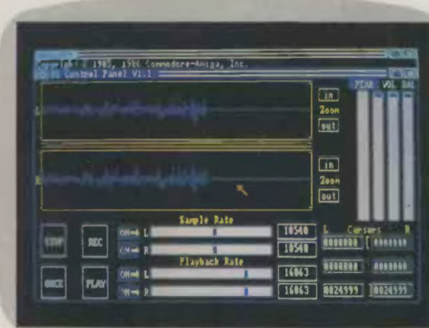
Sophus S5 has two amplitude/time graphs, one for each channel of the stereo sample. The four 'push-buttons' in the left-hand corner operate like those on a cassette recorder
