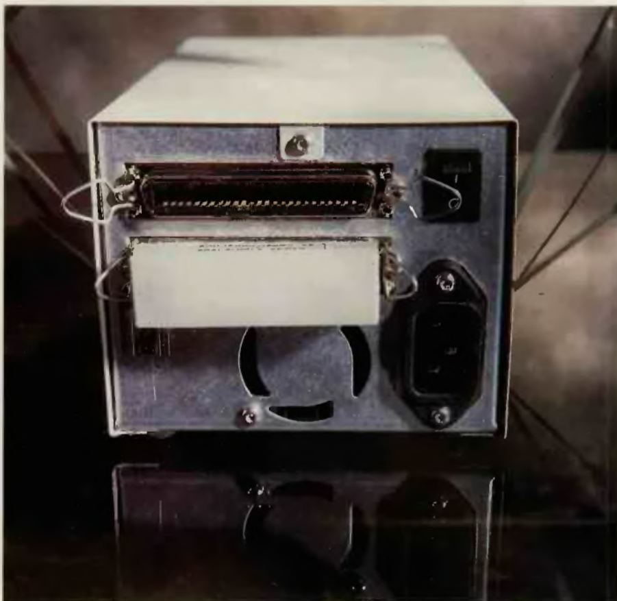
▽ The HP DAT from behind. Extra devices can be connected using the through SCSI connector. A small fan keeps it cool
