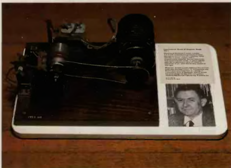
△ An experimental magnetic drum. Early drums were used as main storage; programs could be optimised by taking into account the speed of rotation
