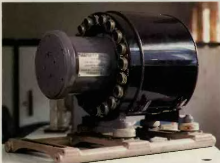
△ An early Ferranti magnetic drum. Today, Conner would get this much store onto a 2.5in disk
