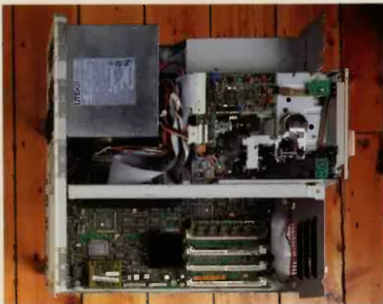
Video RAM is expanded by using an upside-down PCB
