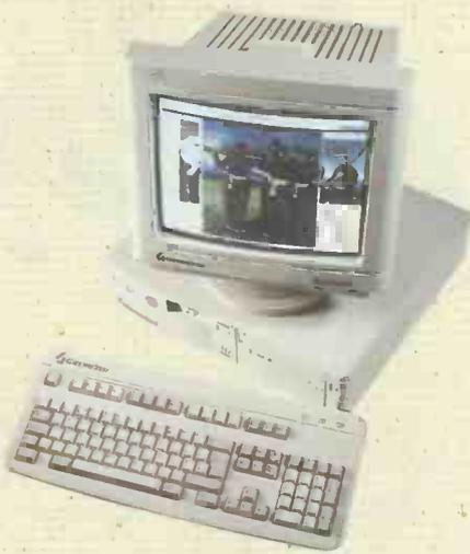
This is the desktop version of Mesh's DX2/66 multimedia machine. Inside, everything is fairly standard with the left-hand side of the box housing the motherboard, processor, and card slots while the righthand side holds the power unit and Sanyo CD-ROM drive. In the centre sits the disk drive with a 730Mb Western Digital hard disk underneath.
