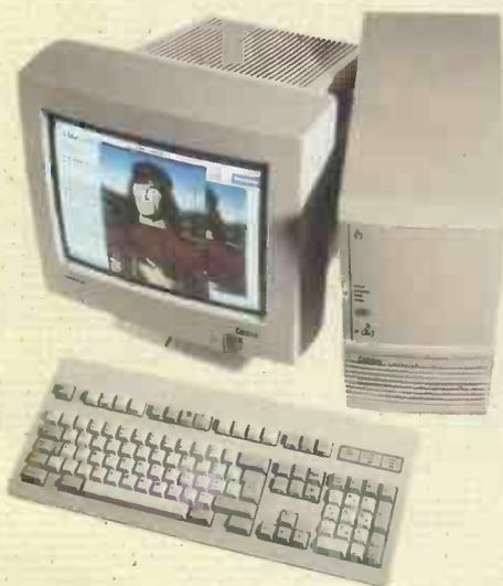
The first thing you notice about this machine is its built-in security features. On the front there's a lockable door which prevents access to the CD-ROM and disk drive. To the left of the drives there's a large power switch and below it are the usual reset and turbo buttons, but there's an extra button which allows you to disable the keyboard before locking the door. These features can be handy, but of course, they won't stop anyone from running
