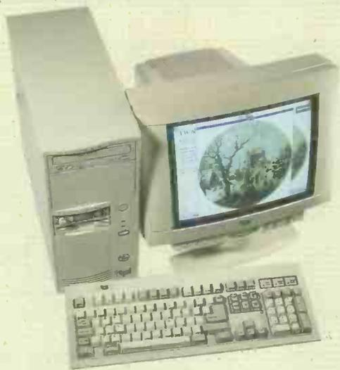
At the front of this machine, believe it or not, there's a graphic equaliser, or more specifically, the Equaliser Amplifier Pro from Platinum. It has seven bands, a volume and balance control, and aims to turn your PC into the full-range, stereo, 60W sound machine that multimedia PCs always promised to be.
