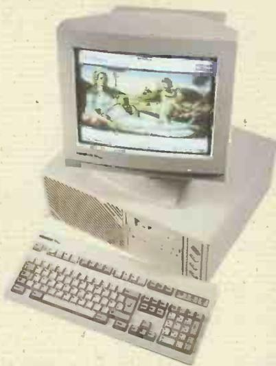
**P**eacock and AST are the only two manufacturers in this group test to submit machines using Cyrix processors. This machine's CPU, though, stands out in another way — it's a DX2/80. According to Cyrix, it offers up to 35 percent improvement over an Intel-based DX2/66 for the same price, which is why we decided to include it here.
