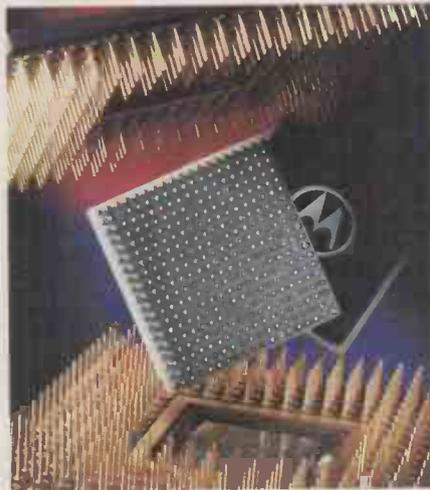
*BGA technology allows more connections per chip*
