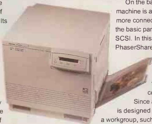
On the back of the machine is a panel for more connections than the basic parallel and SCSI. In this case, it is a PhaserShare Ethernet
