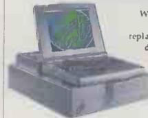
With a docking station on your desk the Voyager becomes a true "desktop replacement". The docking station has two drive bays (1x3.5" & 1x5.25"), three ISA expansion slots (2x full length & 1x 1/2 length), as well as permanent ports for monitor, keyboard, PS/2 mouse, serial, parallel, speaker, microphone and audio line-in.
