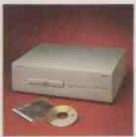
**Philips CDD522 Dual Speed External SCSI CD Recorder** which can record the full range of formats (subject to software used) CD-ROM, CD-ROM XA, CD-I, CD-DA, Photo CD (restricted image sizes) and VideoCD.
