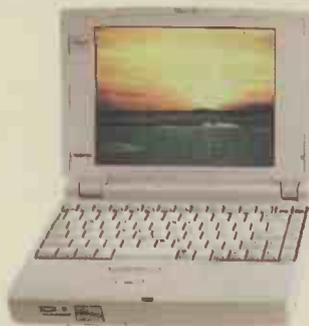
supplier will soon be turning out 11.3in screens in production quantities; because of the way TFT screens and CRTs are measured, 11.3in TFT screens will have almost the same viewing size as a 14in CRT monitor. This TFT can display true colour, or on an external monitor the Chips & Technologies graphics chip can cope with up to 1024 x 768 x 256, thanks to its 1Mb RAM.
