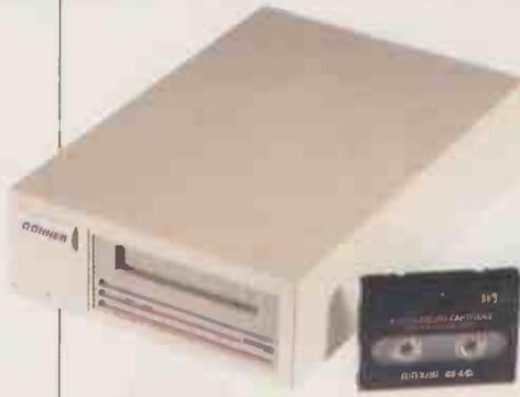
Conner's CTD-8000e, also known as a 4356XP, is a DDS-2 DAT drive. In native mode it can take 4Gb DDS-2 DAT tapes, and can just about double this using hardware compression.
