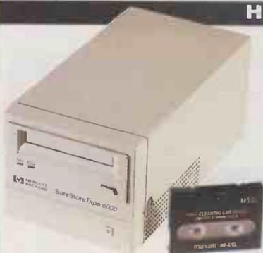
**H**ewlett-Packard does a rather neat line in backup drives using a variety of technologies. We tested the 2000e model from the SureStore range of DAT drives; all are SCSI-2 devices.
