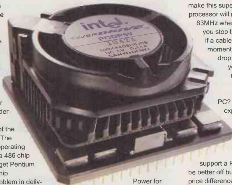
Power for existing fans is drawn from the power supply, either from pins on the motherboard or from a floppy disk power cable. The P24T draws power for the fan directly from the ZIF socket. The fan can be detached from the processor and Intel offers a lifetime guarantee on the fan. Removing the fan reveals three contacts on top of the chip: two of these power the fan and the third provides monitoring of the fan's performance.
