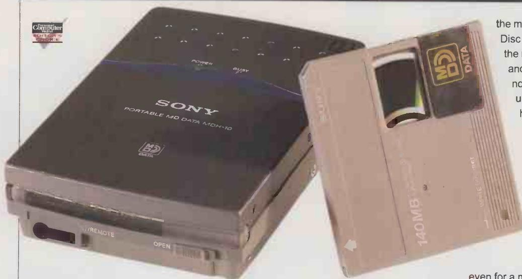
**A**bout three years ago Sony launched its MiniDisc (MD) format, capable of storing 74 minutes of digital audio on a 64mm diameter MO disc. The company managed to incorporate the same audio capacity as a CD, onto the MD using a compression ratio of around 5:1. Uncompressed, the MD media could store 140Mb information and the world wondered when Sony would get round to creating a computer data version.
