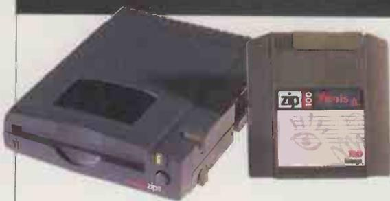
**I**omega describes its colourful ZIP drive as the new floppy drive, although it won't read conventional floppies. Instead, it uses 100Mb cartridges containing a flexible platter. When formatted, the ZIP carts offer 94Mb and cost around £15 each.
