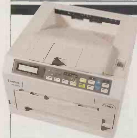
**T**his is the most compact printer of the group, with a tiny footprint that could fit onto almost any desk, and the only printer here to use LEDs instead of a laser.
