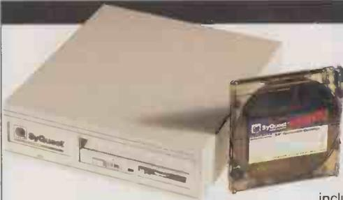
**A**ll SyQuest drives use the same kind of media: the rigid platter of a hard disk, fitted inside a plastic cartridge. When inserted into a suitable SyQuest drive, the combination effectively becomes a hard drive, with similar performance.
