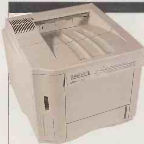
The HL1260 is one of the smaller printers here, compacted into a cube which can take 500 sheets as standard. It is Brother's only workgroup laser.
