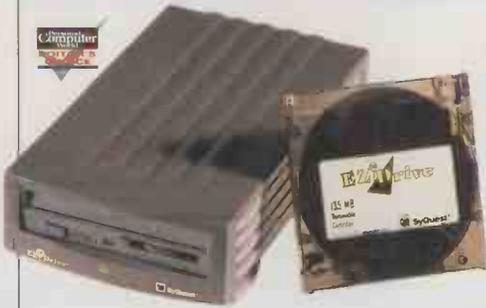
**S**yQuest introduced its 3.5in drives with two models: one with single-sided media 105Mb capacity (now discontinued), and the other, a double-sided 270Mb, reviewed in these pages. The EZ135 Drive is not much more than a remodelled, repackaged and remarketed cross between the two.
