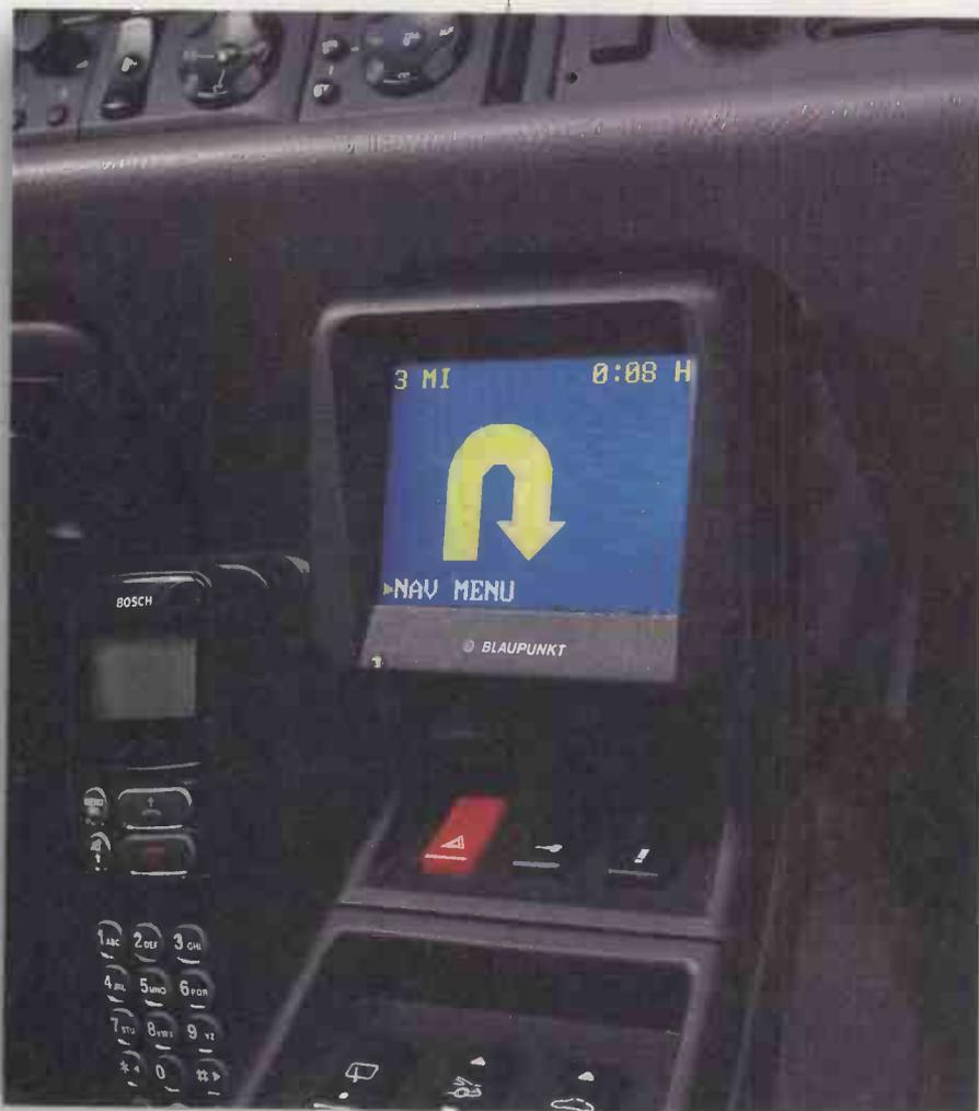
system is the map. The guidance systems only need to direct the computer to the accuracy of one road junction before the map takes over. The GPS locates the car roughly within 25 metres. From here, it can work out the car's position on the map. If you drive out of the area covered by the map, the arrow merely points directly towards your destination. Once you are on the map, the software looks you up.
