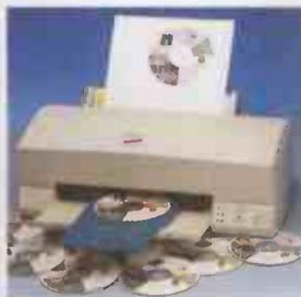
**CopyTrax Printers** - CD-R full colour inkjet printers. Matisse a low PC cost solution and Da Vinci for PC/ Mac. Precision Printing Protocol technology ensures perfect print positioning on the CD-R. Matisse prints 360 dpi to printable CD-Rs in addition to 720 dpi paper printing. Da Vinci prints CD-Rs at 720 dpi & paper at 1440 dpi.
