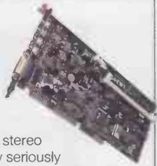
To support these features, the card has a front panel that fits in a 5.25in bay to provide a headphone socket, MIDI and digital I/O. Inside there's a daughterboard connector for an additional synth. The onboard synth/sampler has 6Mb RAM (expandable to 64Mb) and provides up to 64-voice polyphony. DSPs provide real-time digital effects for all audio sources and, in principle, hardware mixing for up to 32 stereo channels.
