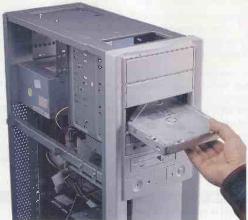
Replacing the hard drive. It's easier to slide the new drive into one of your PC's forward-facing bays. But installing it inside the case, perhaps under the floppy drive, leaves room for extra devices
