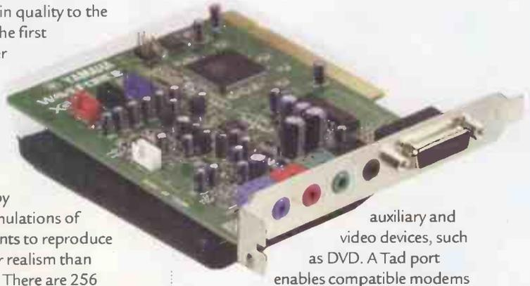
auxiliary and video devices, such as DVD. A Tad port enables compatible modems to be connected to provide two-way telephonic communications. There are connectors for speaker and line output, mic and line input. Audio from the mic input can be routed to the three internal effects buses, including reverb and chorus settings. Bundled software includes a 100-track MIDI sequencer, an audio-file player with 100 classical-music MIDI files.
