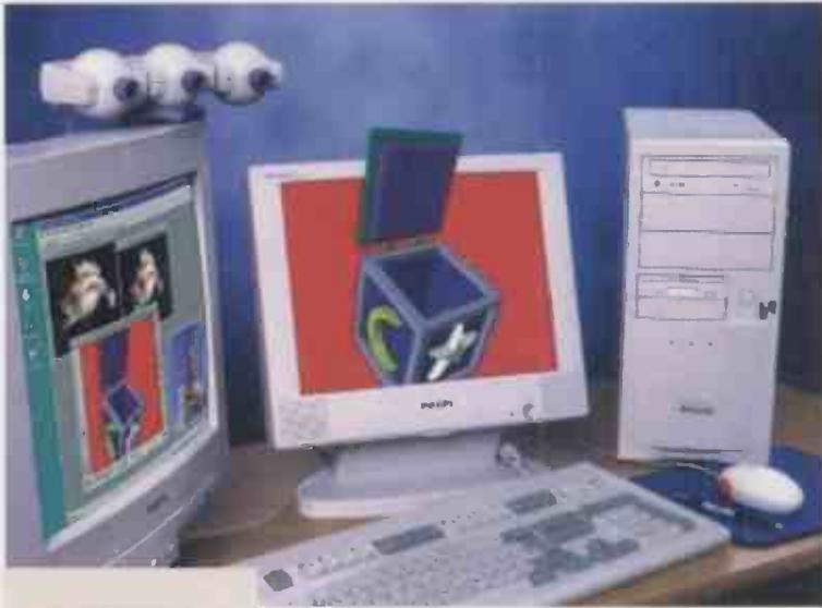
▲ **FIG 1** THE PHILIPS 14.5IN COLOUR 3D-LCD EVALUATION KIT
