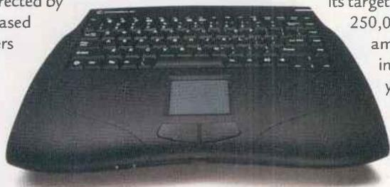
everything is inside a single keyboard, with an output to TV. There is also a VGA connector for optional monitor, a floppy drive, and a 56K modem. There is no hard disk, nor for that matter a C64-compatible cartridge port, but there is a connector for a PCMCIA card unit and an infra-red port for an optional wireless keyboard. You don't get a mouse, but there is a laptop-style touchpad instead.
