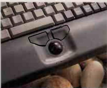
the base unit leaves little space for the wrist rest, making it less comfortable when using the lower keys and space bar.
