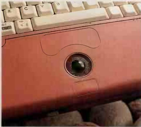
bold markings to differentiate between the key groups. The trackball is quite small but smooth. The large buttons are covered by the rubber surface and work extremely well.
