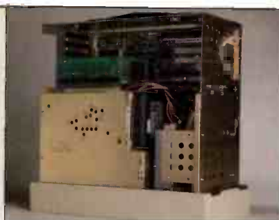
Inside the Colossus CRT case showing integral 9" SVGA colour tube, fitted hard & floppy drives with spare bay, PCI motherboard and expansion slots.
