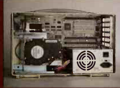
Inside the universal case for Plasma, Dual Scan and TFT models showing Power supply, fitted hard disk with 2 bays spare, Pentium 90 motherboard and PCI/ISA expansion slots.
