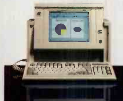
The unique advantage of the Colossus range is the ability to take standard PCI, ISA, VESA and EISA expansion cards.
