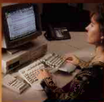
Keyboard split at an angle of 30° with steep roof inclination and optional numeric pad on the left.
