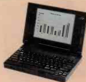
Portable Dock I has standard ports, SCSI, Speakers, one ISA slot, one 5.25" drive bay (suitable for CD-ROM) and a handle. Shown with ThinkPad attached
