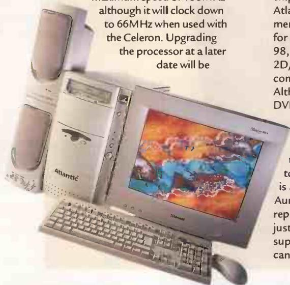
easy, as the motherboard and RAM are ready to run faster and so give a big performance boost. The 6.4Gb hard drive in the Pro 98 is larger than the one in Tiny's system and is adequate for a family PC. There are three PCI slots free.
