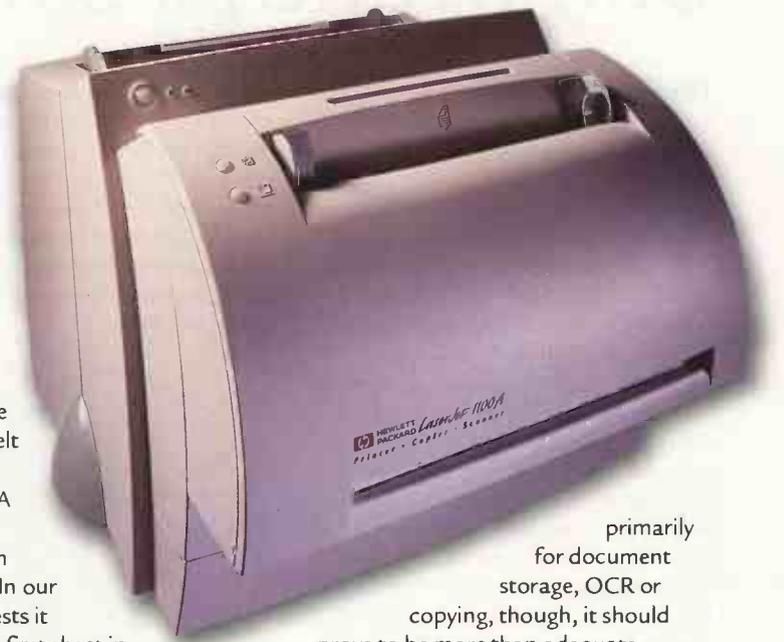
primarily for document storage, OCR or copying, though, it should prove to be more than adequate. Connecting it to the PC allows you to interpolate the optical scanning resolution to achieve 600dpi. A 20-page input hopper allows copying to take place unattended, although without a front panel it is not possible to make multiple copies without the use of the PC.
