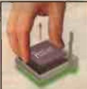
**1** Remove PC cover. Locate CPU/processor socket, release lever and remove CPU.
