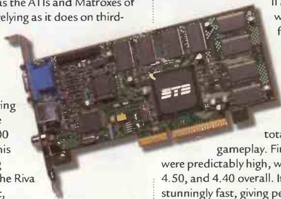
The Velocity 4400 is fitted with 16Mb of VRAM, enough to run a 3D desktop application such as trueSpace at 24-bit, 1,280 x 1,024 resolution with 24-bit Z-buffering.
