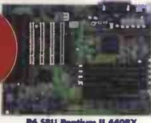
**SUPER P6SBA/S** running at bus speed of 100MHz, supports single Pentium II 400/350/333/300/266/233 MHz processors. P6SBA/S is based on Intel's 440BX chipset, enabling AGP, 100 MHz SDRAM, concurrent PCI, Ultra DMA with 33 MB/s burst data transfer rate, and Wake-on-Lan.
