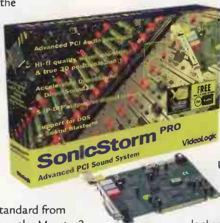
The SonicStorm Pro handles 64 MIDI voices in hardware and the same number of audio voices. As befitting a next-generation sound card, it has a dedicated digital SPDIF output. Unlike the SPDIF output in the SoundBlaster Live!, which is locked at 48kHz, the SonicStorm Pro has a frequency response of 44.1kHz which enables it to output CD-quality audio to a DAT
