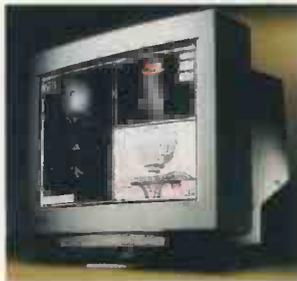
This 21 in Eizo FlexScan T960 offers a 1600x1200 resolution at a refresh rate of 92Hz on a low-reflection flat screen. It packs a USB hub and twin video inputs and costs £959 ex VAT.
