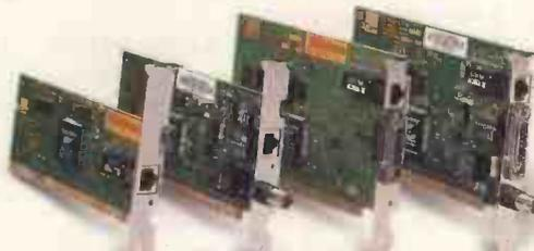
Parallel Tasking technology allows adaptors to overlap tasks & increase performance. The adaptor starts writing the first portion of a packet onto the network, while it is still reading the last portion of the packet still in the adaptor's memory - simple!
