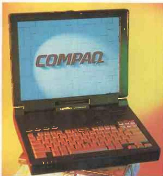
and suspend operation. The lid houses the screen, a microphone and two speakers that provide excellent sound for a laptop.
