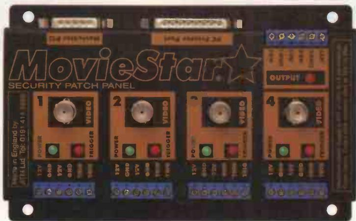
Connect standard alarm sensors to these screw terminals in order to trigger AVI movie recording to hard disc. Devices such as PIR (Passive Infra Red) detectors, invisible beams, pressure mats and door & window contacts are suitable.
