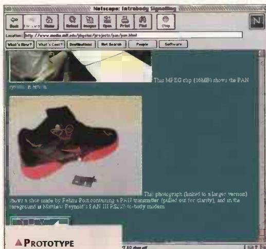
▲ **PROTOTYPE INTELLIGENT FOOTWEAR, BY MIT'S REHMI POST. CONTAINS SOFTWARE AND BOARD TO CREATE A 'PERSONAL AREA NETWORK' (PAN), WHICH CONFINES NETWORK ABILITY TO THE WEARER AND ANY DEVICE HE OR SHE INTERACTS WITH. IN THIS WAY A DOOR, FOR EXAMPLE, COULD BE PROGRAMMED TO OPEN ONLY TO THE WEARER OF A PAN-ENABLED WEARABLE DEVICE**
