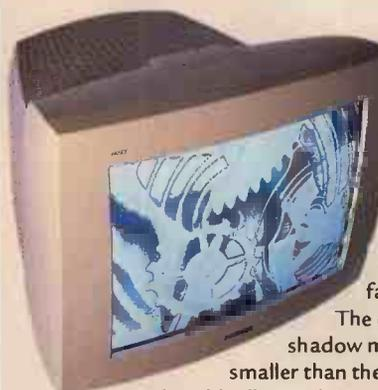
The 447XS has all its controls on the right-hand side, resulting in a reduction in height and making the unit look very squat indeed. It works pretty well though, with the controls falling naturally to hand. The display itself is a shadow mask and slightly smaller than the rest, with a 15.7in viewable diagonal. In use, colours are unusually vibrant for a shadow mask and the display is crisp with no signs of ghosting. Four USB ports nestle in the base.
