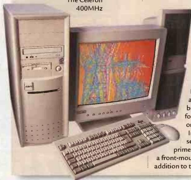
processor produced lower benchmark scores than the PII 400s in this test, partly because the Celeron front-side bus only runs at 66MHz rather than the 100MHz speed of the PII 400s.
