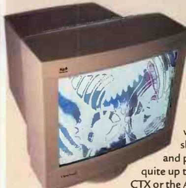
This is one of the more expensive 17in displays in the test but the PT775 is backed by very good performance. It displayed excellent resolution, colour alignment and focus, which add up to a very sharp picture. Vibrancy and purity of colour weren't quite up to the standard of the CTX or the ADI, though. There's no USB support but there are both D-SUB and BNC video inputs. The ViewSonic should definitely be on your 17in shortlist.
