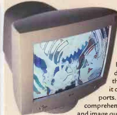
The 795SC is a little uninspiring to look at and produces a fairly uninspiring display, too. It's a shadow mask unit with the screen curved in both the horizontal and vertical directions. There's just the one D-SUB input and it doesn't have any USB ports. The OSD is comprehensive and easy to use, and image quality is good but not remarkable. Horizontal resolution wasn't perfect and colour convergence was slightly awry, but the LG would make a good, basic office display.
