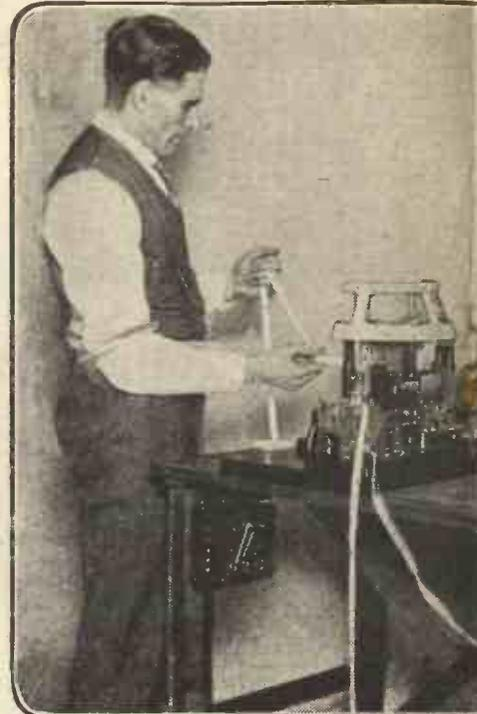
Using the Creed system, it is possible to print messages. This illustration shows the wireless messages on perforated paper being printed by the printer, whence they pass on.
