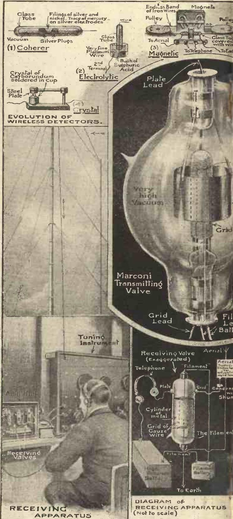
Our illustration shows the wonderful progress made in wireless since the early days of the left; are to be seen the detectors, which the wonderful electron valve has practically supplanted. The day of the coherer and the magnetic detector is in the past. The transmitting valve used for continuous wave and telephony. This type of valve is again speaking into a wireless microphone.
