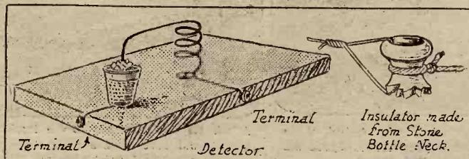
Next take the neck of a broken ginger-beer bottle (being careful not to cut yourself), and tie a piece of rope or string round it by which you can attach it to your aerial pole or the highest point of the house. Thread the end of the remainder of your enamelled wire through the neck, keeping rope and wire from touching. This will make quite a good insulator. If desired, you might buy one which would look nicer.
