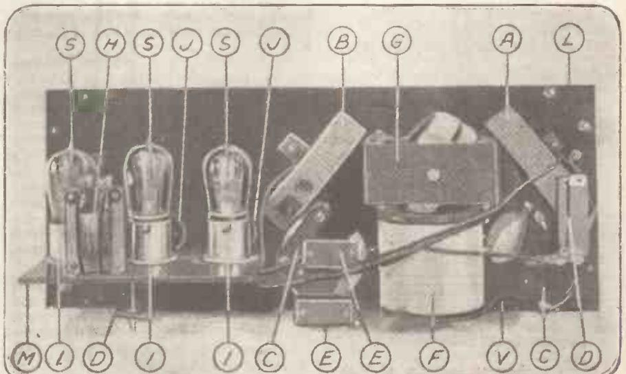
Fig. 1.—The various items that are required in the assembling of this Armstrong-circuit set are illustrated in this diagram. Note that the coil F and the variometer G are placed in inductive relation to each other. The regeneration in the first valve is controlled by the variometer.
