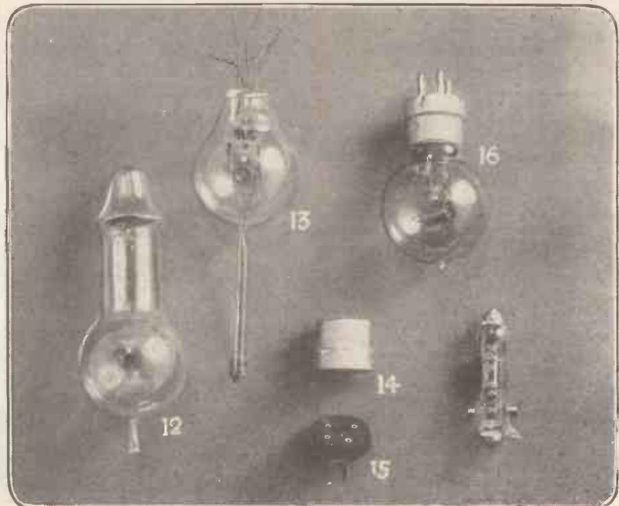
The valve nearing completion: The last phases in its construction.
