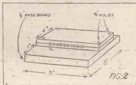
you have two slotted sections exactly the same size. Place the slotted sides face to face squarely, and stand them upon the other sheet of ebonite (6 by 3 by  $\frac{1}{4}$  in.) which forms the baseboard. If they are placed in the centre there should be an inch clearance at each end of the latter, and the whole should appear as in Fig. 2.
