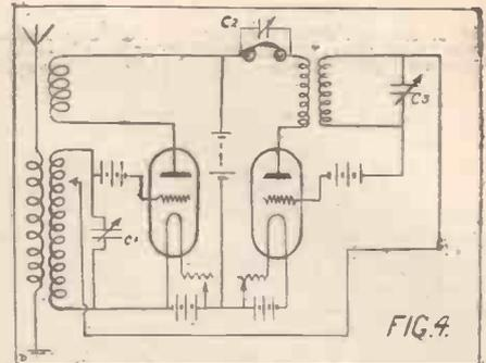
Fig. 4.—This diagram illustrates the method of obtaining super-regeneration by varying the damping of the first tube circuit with respect to regeneration. The set described in this article uses an adaptation of this method.
