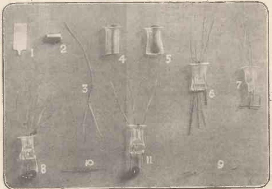
The various parts of the valve before assembling.
