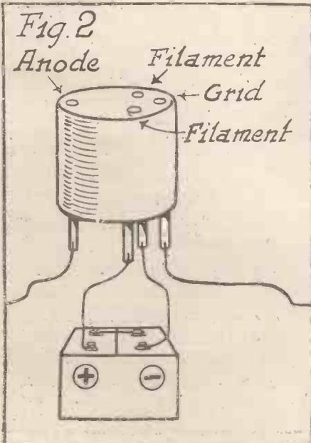
plate; the two pins marked  $F_1$  and  $F_2$  are connected to the two ends of the filament wire. Sometimes the valve will have the cap lettered showing which pin goes to which electrode; sometimes the pin going to the anode is indicated by the letter A or P. The pin immediately opposite is the grid, while the other two are the filament pins.
