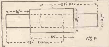
not to disturb the position of the foil, each of which should be directly over the next below, the same rule applying to the tabs, or tails. (There should be 2 tabs one way, and 3 the other.) Drill four holes at the corners of the ebonite sheets, and countersink one set sufficiently deep to take the bevel of the wood screws. These parts should now be placed on one side until they are required for mounting on the panel of the receiver.
