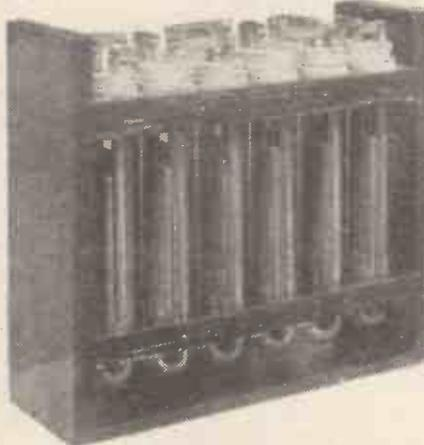
A "Chloride" H.T. Battery, with glass test tube containers.
