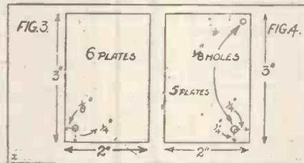
through one corner, the centre of which should be  $\frac{1}{8}$  in. from one edge and  $\frac{1}{4}$  in. from the other (Fig. 3). Now clamp the remaining five plates, and drill a  $\frac{1}{8}$ -in. hole through each corner on the 3-in. side, the centre to be  $\frac{1}{8}$  in. from each edge.
