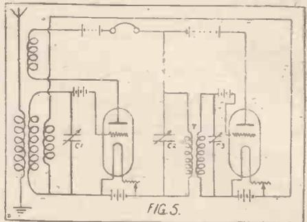
Fig. 5.—This circuit diagram shows how super-regeneration may be obtained in still another way—by varying the amount of regeneration with respect to the damping of the input circuit of the first tube.
