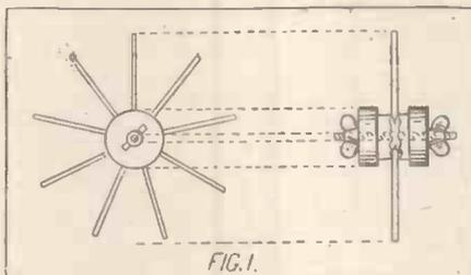
The next consideration is the number of spokes, which is determined by the size of wire with which the coil is to be wound. If thick wire is to be used on a small-sized coil nine spokes are sufficient, but this should be increased to eleven or thirteen for larger sizes employing finer wires. The chief point to remember is that the number of spokes must be odd, as otherwise the coil will not take up a basket formation; in fact, it will be impossible to wind it unless this rule is observed.
