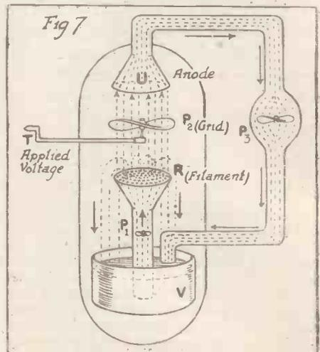
main propeller H revolving at the same speed. The distance between U and R weakens the suction effect on water emerging from the rose R; but the propeller  $P_2$ , being quite close to R, has a very big effect on the quantity of water sucked up into the funnel U.
