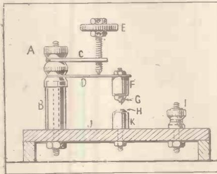
The parts F and K are two crystal cups. These can be bought of any wireless dealer, or can easily be made from old brass cartridge cases.
