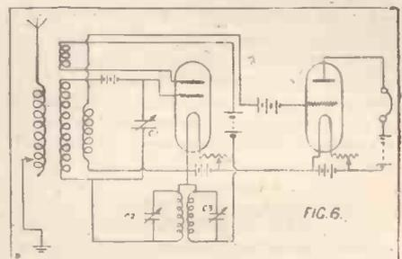
Fig. 6.—How super-regeneration may be obtained by varying both the damping and the regeneration with respect to each other, keeping the proper phase relations.
