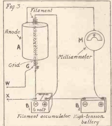
possible to explain here all the reasons why the three-electrode valve may be used as a detector or amplifier; it is only proposed to give a very brief theoretical description. It is found that if a positive potential is applied to the grid of a three-electrode valve, the electron current from the filament to the anode and round the anode circuit is increased, whereas if a negative potential is given to the grid the normal steady current round the anode circuit is decreased.
