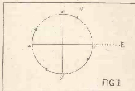
This merely means that, with reference to any particular transmitting station, there are two maximum and two minimum positions for each frame aerial. Reference to Figs. 2 and 3 will make this clear. Fig. 2 shows the plane of a single loop aerial. The line with the arrows, drawn across the plane, shows the two directions from which maximum signals could be received. Similarly, if we imagine the transmitting station at E, maximum signals will be received whether the side AB or CD is nearest to it.
