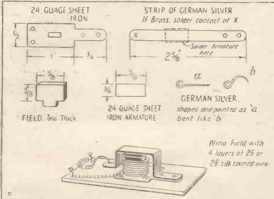
Making a Small Testing Buzzer.
