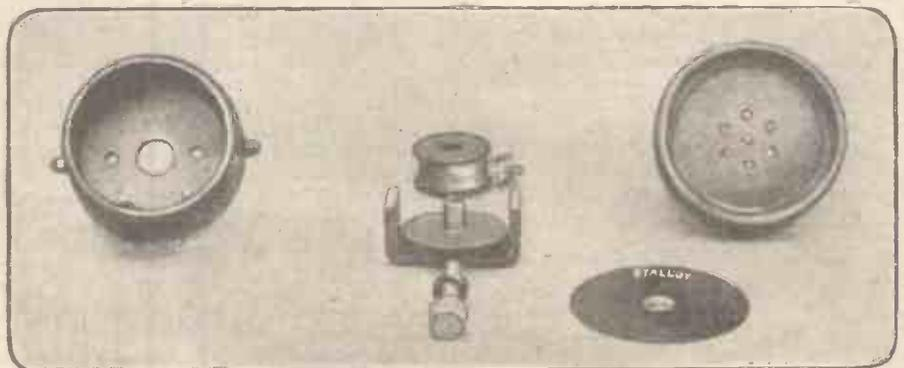
Component Parts of the Watch Receiver Telephone.
