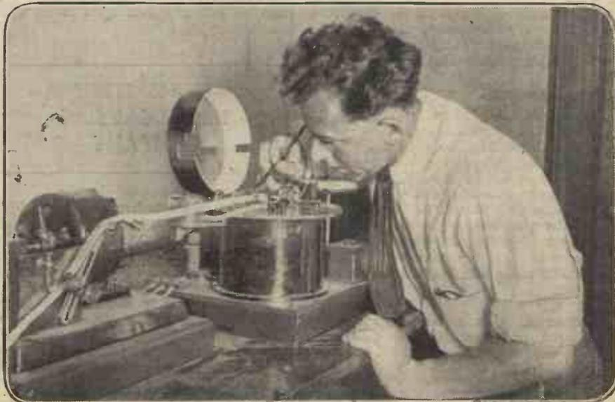
A high-speed ink recorder of radio signals. It can record 200 words a minute.
