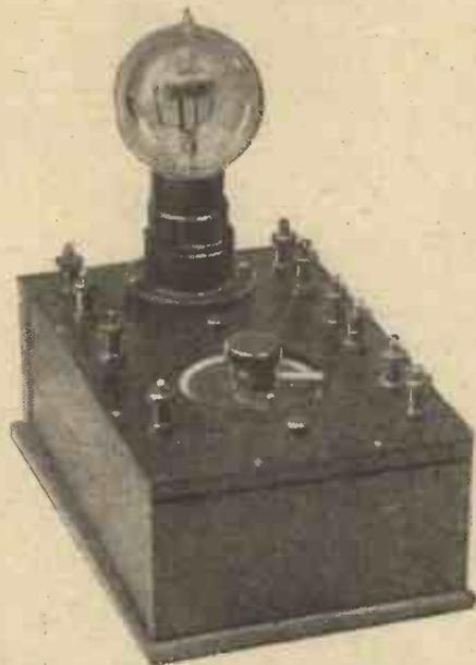
The Thermionic valve, mounted on panel and ready to wire up to a set.
