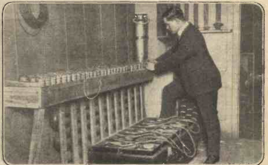
The Battery Supply Department for Radio use on an American Express Train.
