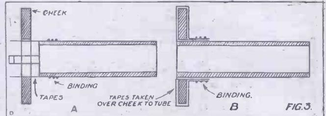
When this is done the core may be inserted in the bobbin, the first binding wire should not be removed to prevent the wires fanning out, but all the others should be removed as the core is inserted. When the core has been pushed through the bobbin, the first binding wire may be removed and the core adjusted to project equally either side.
