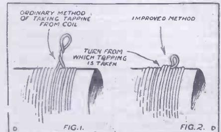
winding of the coil, bend the tapping down flush with the former and wind the following two or three turns over the base of it. Then raise the loop of the tapping up again and continue winding the coil until it is desired to make a further tap, and so on, until the coil is completed.
