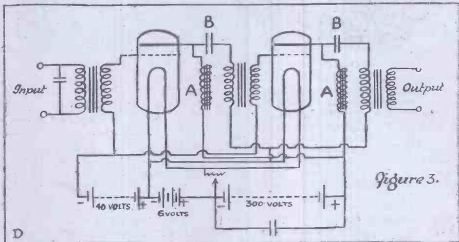
them down. It is best and cheapest in the long run to install a plate battery of small accumulators, or failing that, current from the mains or from a motor generator may be used, a system of choke coils and condensers being used to get rid of the hum. The owner of an ordinary note magnifier can easily convert this to a power amplifier,
