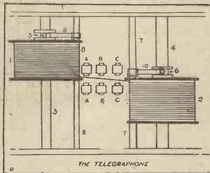
word, but it does so in a semi-permanent form. That is to say, the magnetic record will remain available until it is deliberately effaced, which, however, can readily be done by passing the wire across the poles of a second magnet. Once it has been so "cleaned," the wire is ready to receive another "impression" which, in turn, can be destroyed, and so on, the same piece of wire being used as often as desired.
