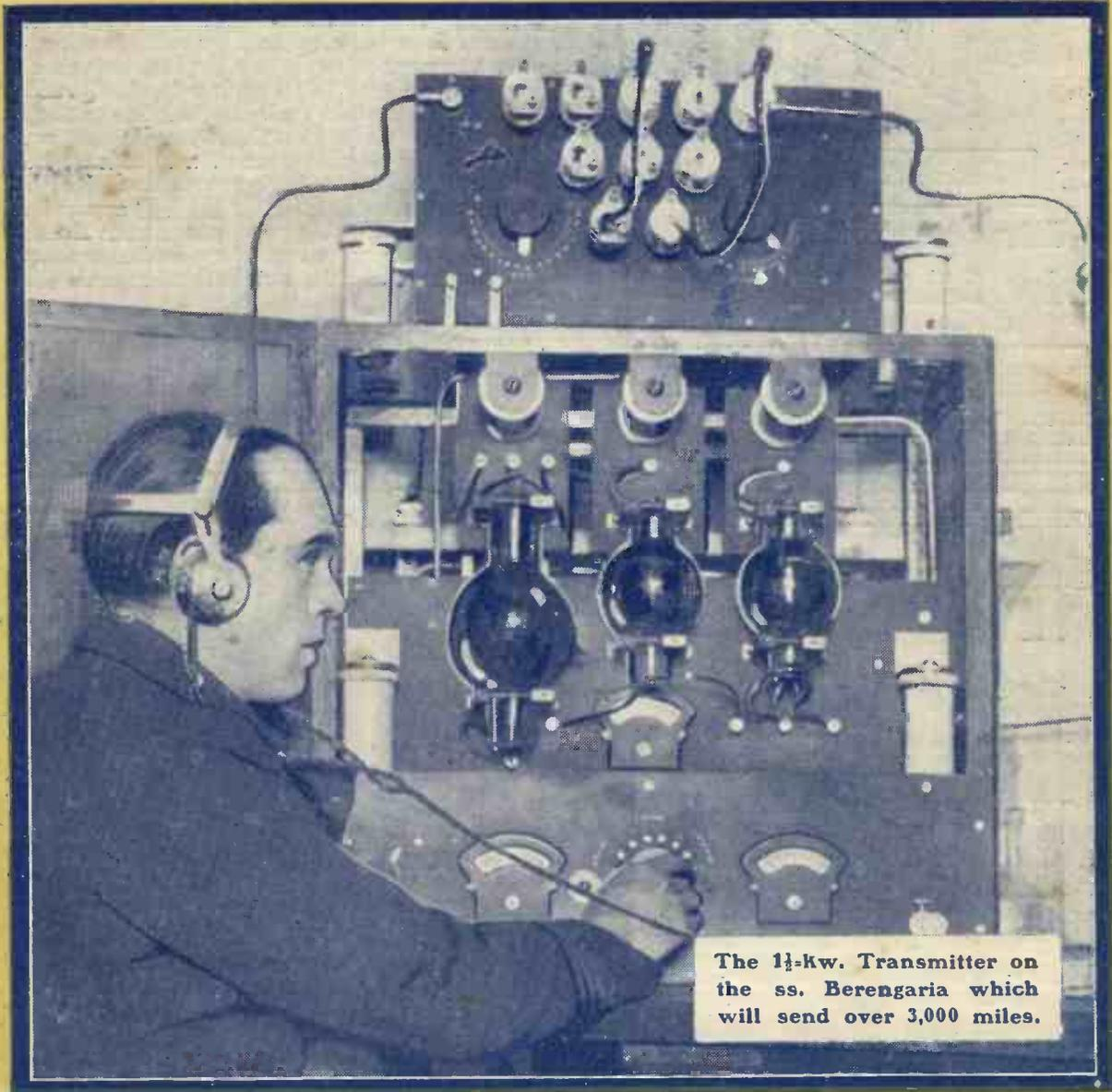
The 1½-kw. Transmitter on the ss. Berengaria which will send over 3,000 miles.
