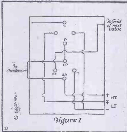
Fig. 1 shows the wiring of a typical high-frequency panel, the sockets at the top of the panel being for the valve and the lower ones for plug-in transformers. From this it will be seen that the plate of the valve is connected to one side of the primary of the transformer, the other side being connected to + high tension; across these two is a variable condenser.
