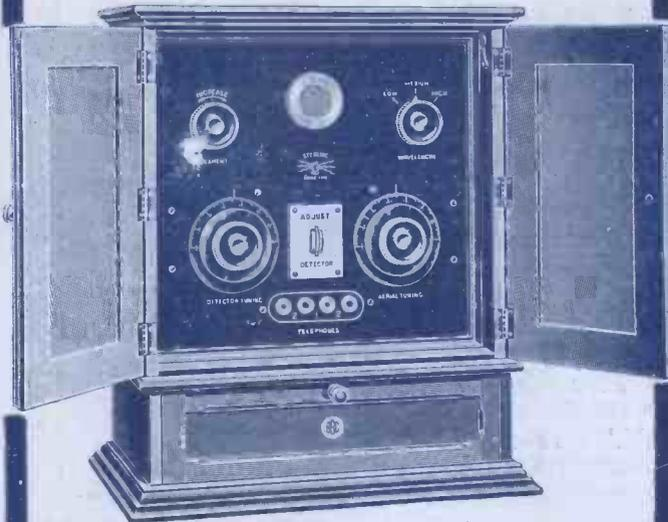
This unique Instrument receives telephony up to 150 miles, is variometer-tuned and has a wave range from 280-2,800 metres.
