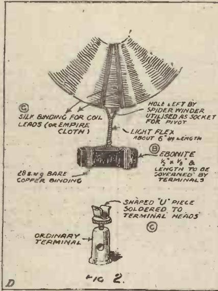
The coil pivots are made from  $2\frac{1}{2}$  in. lengths of 8 in. ebonite knitting needles, pointed each end and one end serewed into the centre of each strip at the point indicated (see Fig. 1). These rods are supported by brass brackets  $1\frac{1}{2}$  in. by  $1\frac{1}{2}$  in. by  $\frac{1}{16}$  in. thick, holed to receive the strips and screws for fixing at A, Fig. 1.
