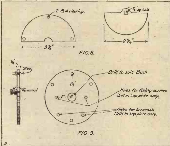
suit the rods and terminals available. The terminals and studs should be tapped into the end plates as shown, so that the top ebonite end plate will be flush with the panel when mounted.
