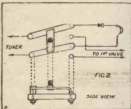
then simply push over the switch and light the filaments. Of course, this type cannot always be used as, in the act of changing over, the switch arms each touch two contacts instead of one, finding sometimes a new path for the H.T. current with disastrous results. In this case an obvious remedy is the provision of two extra "dead" studs in addition to the four studs in use.
