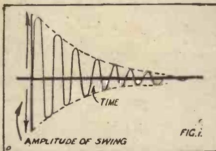
Fig. 1 shows the manner in which the oscillations die away. It will be seen that the time of swing is the same all the while, it is only the amplitude which changes. An exactly similar phenomenon takes place in
