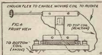
4 in., should be obtained, and the mount with brass plug fixed firmly on to the ebonite on the top of a small piece of ebonite, about  $\frac{1}{4}$  in. to  $\frac{3}{8}$  in. thick, the same size as the mount, in order that the bottom tuning coil may be clear above the surface of the panel, Fig. 3.
