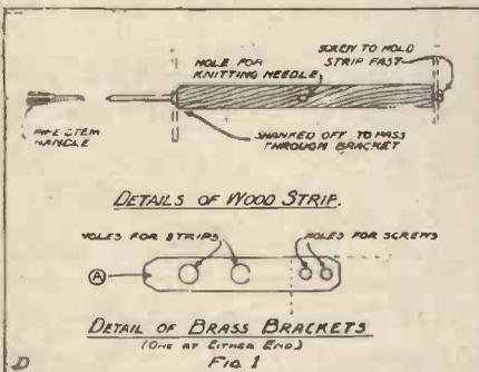
The tuner consists of three small strips of ebonite or wood—the writer used meat-skewers with pieces of a disused pipe-stem as knobs—about  $\frac{3}{8}$  in. square, the length being governed by the width of the tuner plus desired length of the extension handles. It is desirable to keep the outer one longer than the inner one to facilitate manipulation, and it should be at least 4 in. longer than the tuner to minimise body capacity effects.
