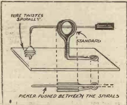
any point in a few moments, and, at the same time, is extremely simple to make. The drawing shows clearly the nature of the construction, which consists of a standard formed out of a piece of brass or G.S. wire, a helix being formed at the top of two or three turns for the various points to be pressed in at will. The spring shaped cup should be made slightly spiral, allowing for a better grip of the irregular shape of the crystals.
