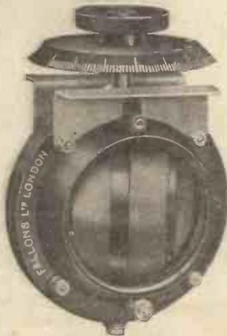
Inside winding, suitable for "broadcast" reception on any P.M.G. Aerial, extraordinary close coupling ensuring large tuning range. On a 30 ft. indoor aerial the maximum wave-length exceeds 420 metres, and the minimum on a 100 ft. aerial is below 350 metres. The maximum on a full-size outdoor aerial is 700 metres, and the minimum on a 30 ft. is 200 metres. Inductance, the highest possible—95 to 1. Metal feet can be adjusted to four different positions.
