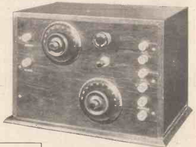
A front view of panel of the Super-Selective Receiver. An L.F. amplifier can be added, but tends to cause great instability unless separate batteries are used.
