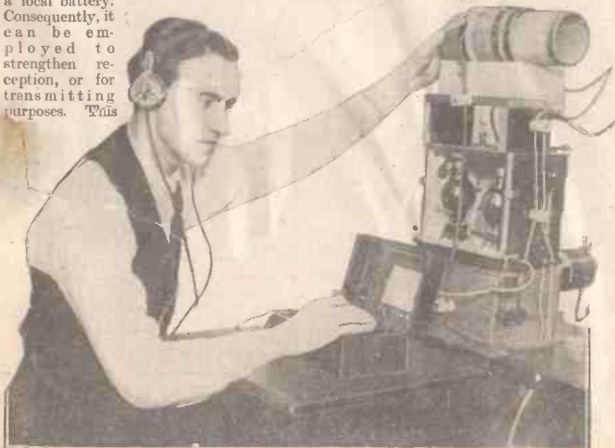
An operator at the Nash Point Station adjusting the wave-length of the C.W. sets by means of a wave-meter.
