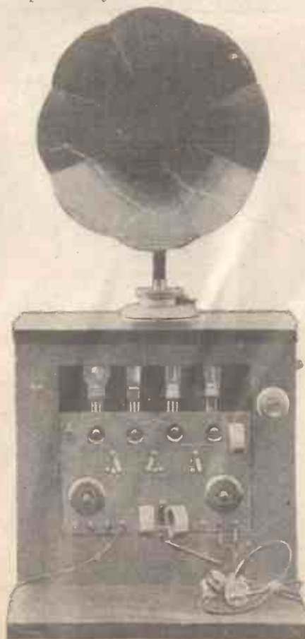
A 4-valve set (1 H.F., det., 2 L.F.) made by Mr. L. Hook, of the Streatham Radio Society. WGY and all B.B.C. and many Continental stations have been heard.
