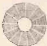
Low self-capacity, accurately calibrated, self-supporting without shellac or wax. Give great selectivity over all wavelengths. Set of 5 coils with instructions 2/6 No. 6 (Daventry) - - - - 1/6
