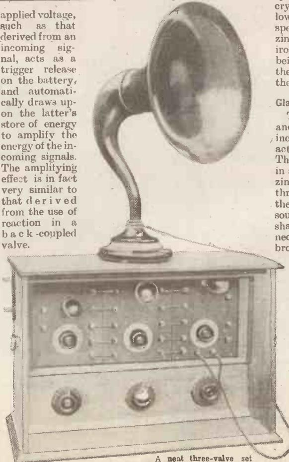
A neat three-valve set (comprising detector and 2 L.F. stages) built on the unit system by Mr. W. Blackledge, of 321, Tonke Moor Rd., Bolton.
