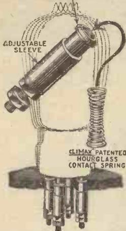
**CLIMAX ANTI-MICROPHONIC VALVE SOCKET** is made on an entirely new principle. The valve floats on metal springs. Each separate socket contains a patented hour-glass contact spring which is truly anti-microphonic and at the same time makes excellent electrical contact.
