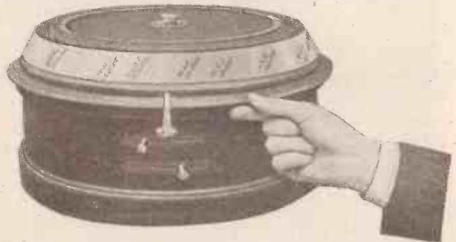
Fig. 2. A "No-dial" Receiver, which contains 5 valves, and is tuned by rotating the lid.
