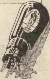
The Scissor Switch in the base of the Valve controls 3 filaments. With the switch closed, any one filament can be used, leaving 2 in reserve. Open the switch, placing 2 filaments in parallel and the Valve is at once a POWER AMPLIFIER.
