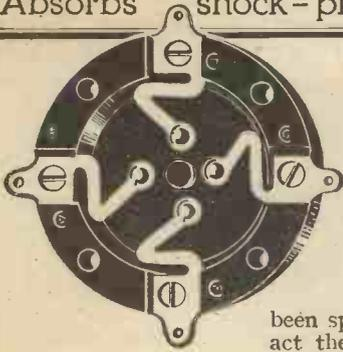
Valve sockets and springs are locked together by a mechanical process, making a definite and permanent connection. Bakelite mouldings, nickel silver springs and phosphor bronze valve sockets. Nickel plated.
