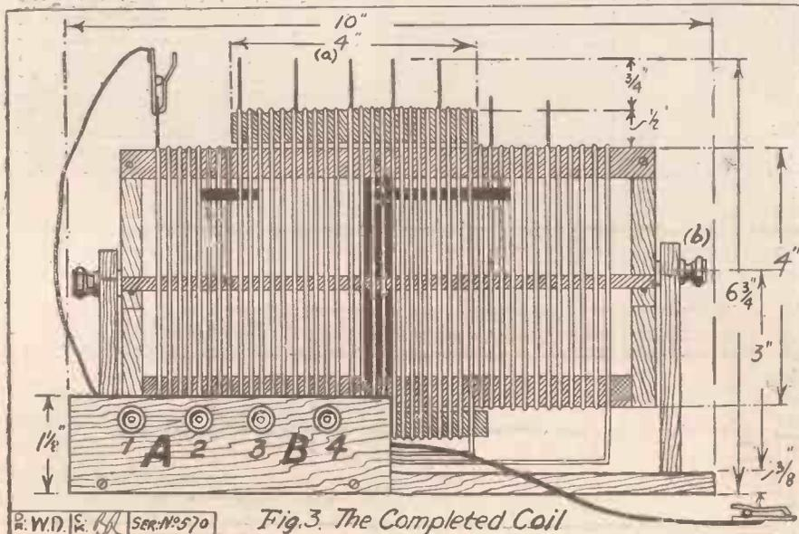
Fig. 3. The Completed Coil
