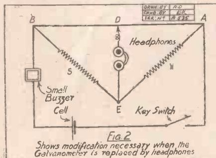
connected as shown, D being a sliding contact which can be made anywhere on the metre wire. The galvanometer will register a current for all positions of D, when the key is pressed, except one.
