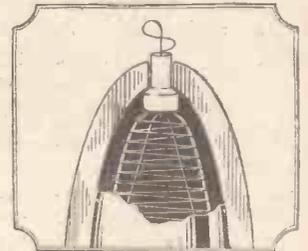
Observe how the seonite insulator securely aligns and holds in their correct relative positions, the filament, the grid and the anode. Through the centre of the insulator will be seen the fine wire which supports the filament and safeguards it against shocks.
