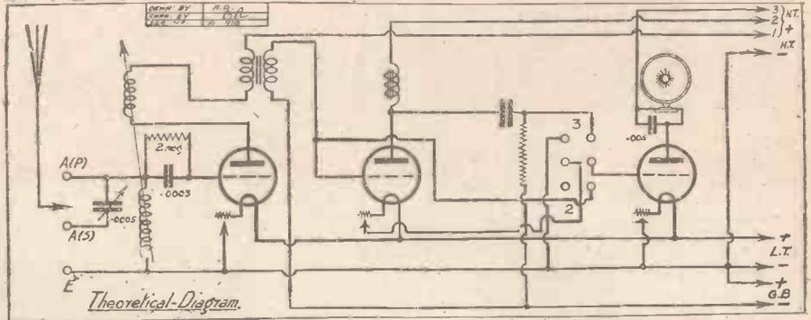
A similar group of impedances should be used if 2 volt or 4 volt valves are employed, and as separate H.T. plugs are provided for each valve and grid bias is included for the last two, each valve may be
