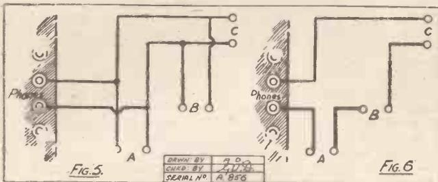
It is very simple. The aerial terminal of the set is connected via a fixed condenser to the loud-speaker extension circuit. That is all there is to it, but it should be noted that the choke and condensers are essential to this system.
