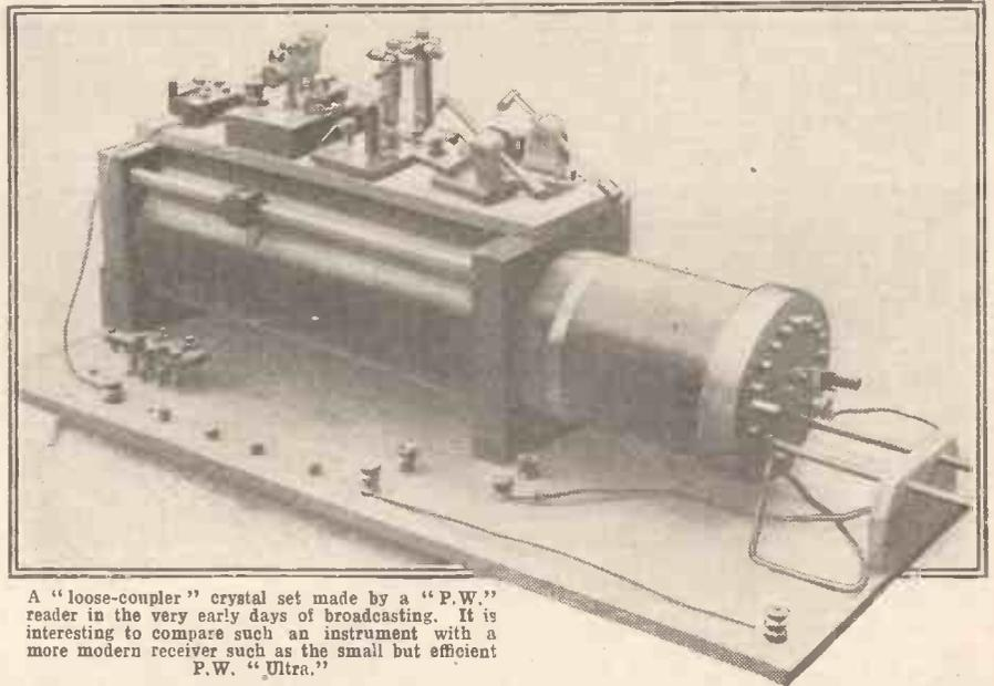
A "loose-coupler" crystal set made by a "P.W." reader in the very early days of broadcasting. It is interesting to compare such an instrument with a more modern receiver such as the small but efficient P.W. "Ultra."
