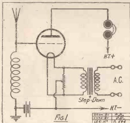
and bring the grid connection to the slider. If the grid connection were taken to one side of the filament there would be a loud hum in the telephones, because the voltage at that point of connection would vary from max. positive to max. negative.
