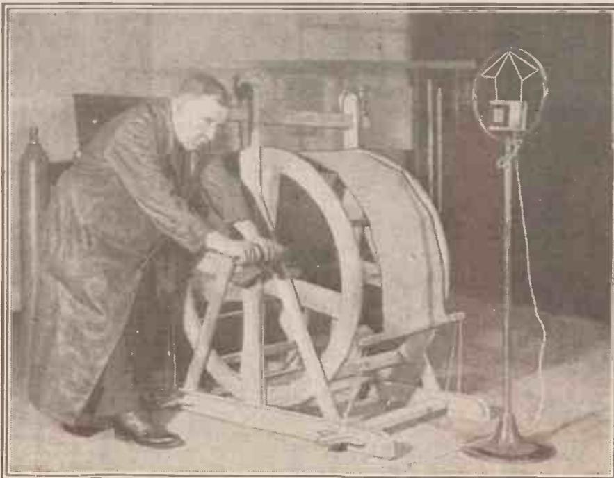
Fig. 4. This machine produces the sounds of anything from a gentle breeze to a thunderstorm.
