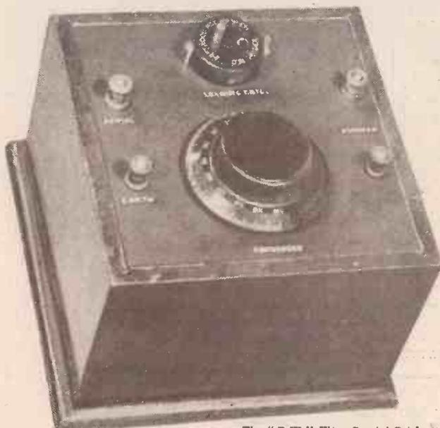
The "P.W." Ultra Crystal Set in its completed form but with loading coil removed.
