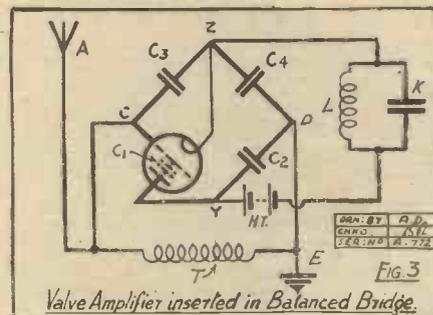
avoid this trouble, steps are taken to completely dissociate the grid and plate circuits.
