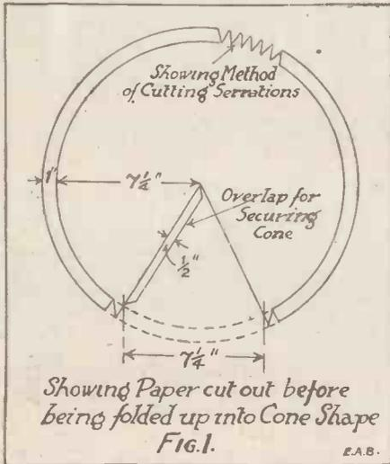
regarding comparative tests. The cone shape is a better reproducer, generally, than the pleated type, and the best average diameter for the cone is in the neighbourhood of 10 in.
