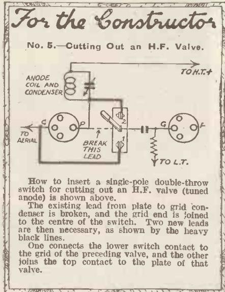
How to insert a single-pole double-throw switch for cutting out an H.F. valve (tuned anode) is shown above. The existing lead from plate to grid condenser is broken, and the grid end is joined to the centre of the switch. Two new leads are then necessary, as shown by the heavy black lines.
