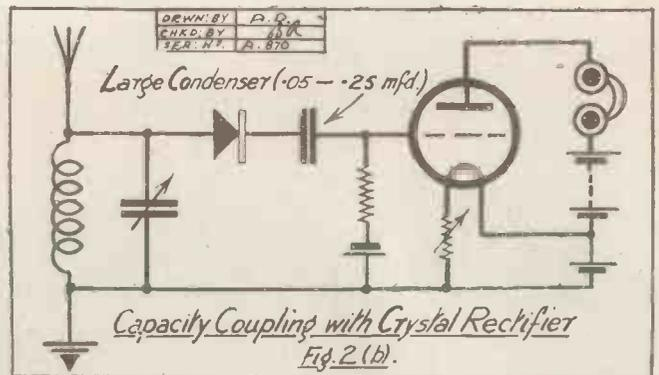
coupling following the crystal is generally negligible, the writer's predilection is for the latter for local work, and for the Sharman for distant stations. But, if the signals are not "boosted up" by reaction the circuit of Fig. 1 (direct coupling), is often very satisfactory, even at quite respectable ranges.
