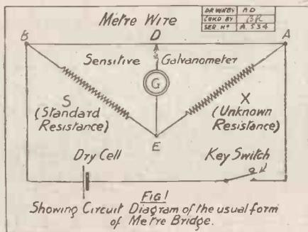
As usually employed, this instrument involves the use of a delicate galvanometer, sensitive to currents of 1 micro-ampere, also a set of standard resistances. It is possible to dispense with the galvanometer, using instead a pair of headphones, which are just as sensitive; and if one or two standard resistances are purchased the rest of the set can easily be made. The instrument itself is also easy and cheap to make.
