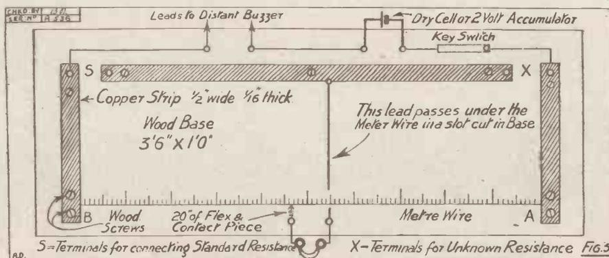
D is varied until this position of "balance" is found. We then have the following relation between the various resistances in the circuit:
