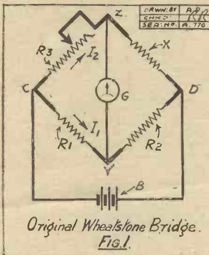
diagonal of the square, and a sensitive current indicator, such as a galvanometer, G, is connected across the other diagonal. The resistance  $R_3$  is made variable, as indicated by the sliding contact.
