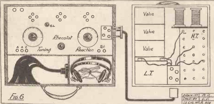
Connection between the batteries and the set can be made by a cable of flexible wires fitted at each end with a plug having a suitable number of contacts at each end, say two for L.T. and two for H.T. The connections of the plug sockets in the receiver and battery cases will be obvious. A suggested design for a receiver on these lines is given in Fig. 6.
