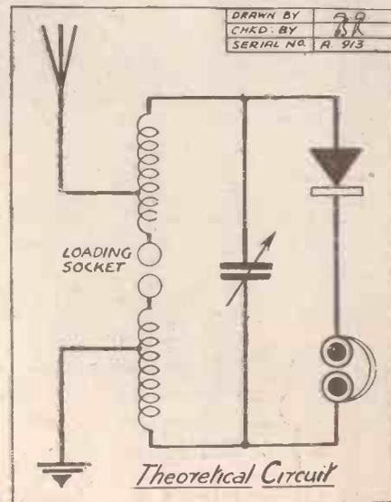
disadvantage of requiring two tuned circuits, one attached to the detector, and the other attached to (and partly consisting of) aerial and earth. Two separate tuning controls are necessary, so in order to obviate this disadvantage, the method known as auto-coupling was evolved.
