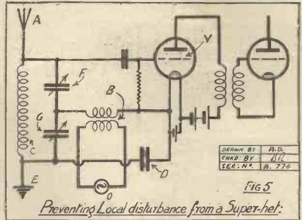
for a true balance is that the capacity of D should equal that between the grid and filament. Once this balance is struck, the aerial circuit is dissociated from the local input coil, B, and any H.F. energy flowing in this coil cannot be communicated to the aerial.
