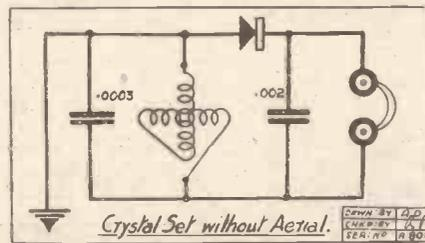
tube variometer crystal set, which I considered very inefficient. One day I put a fixed condenser, .0003 mfd. in parallel with the variometer, and I found that I could receive 2 L.O. fairly well, using only an earth connection. (See diagram.)
