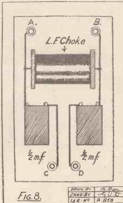
A and B should be connected to the 'phone or loud speaker terminals of the set, and the extension leads to C and D. The inclusion of such an instrument not only makes the wiring easier and safer, but actually improves reproduction, more especially in cases where the H.T. battery is on the downward path] of deterioration.
