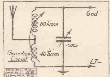
without altering the existing lay-out, a variometer was made in which the 40 turns became the rotor and the 60 turns the stator; the .0005 variable condenser was, of course, still used. In this form it gave very good results and well repaid the time and material used in making it. Should a two-coil holder be used, the wiring should be arranged so that the direction of the coils is the same.
