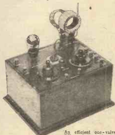
An efficient one-valve DX receiver constructed by a reader of “Popular Wireless.”
