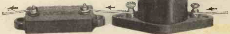
Fig. 2.—A fixed condenser and an H.F. choke joined up in series. The arrows indicate a direction of current flow.
