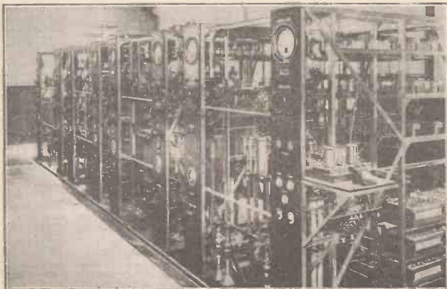
The transmitting gear used at Bodmin for the Canadian beam service, 1925-1926.
