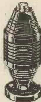
The new **MH** H.F. Choke is scientifically designed to deal effectively with both long and short wave frequencies. With an inductance of 60,000 microhenries, negligible self capacity, and a D.C. resistance of 130 ohms, it is ideal for all purposes.
