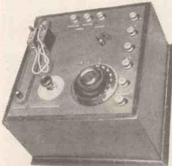
The coil holder and the tuning control—on the left and right respectively—are clearly shown in this illustration.
