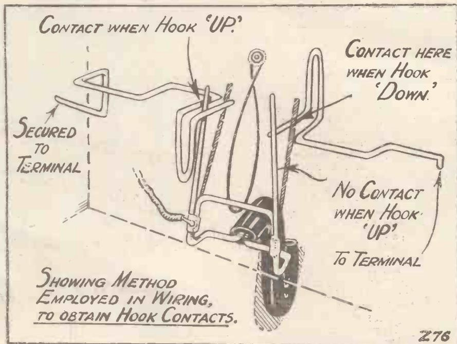
This picture shows in detail the essential mechanism of the "Stethocrys," which is described in the three preceding pages.
