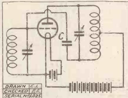
Therefore the valve will be unstable as an amplifier, and liable to self-oscillation unless this feed-back can be counteracted.
