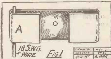
of the strip, it is a good plan to press the pieces together (using pliers) over a bit of 18 S.W.G. wire inserted at the points marked A. This gives a certain springiness to the clip when the wire is removed.
