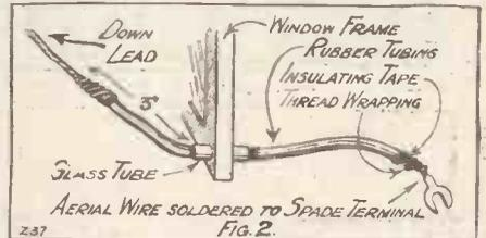
insulated portion of the aerial with the layers exposed for the sake of clearness.
