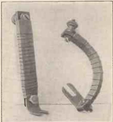
Fig. 5. Two forms of home-made resistors.
