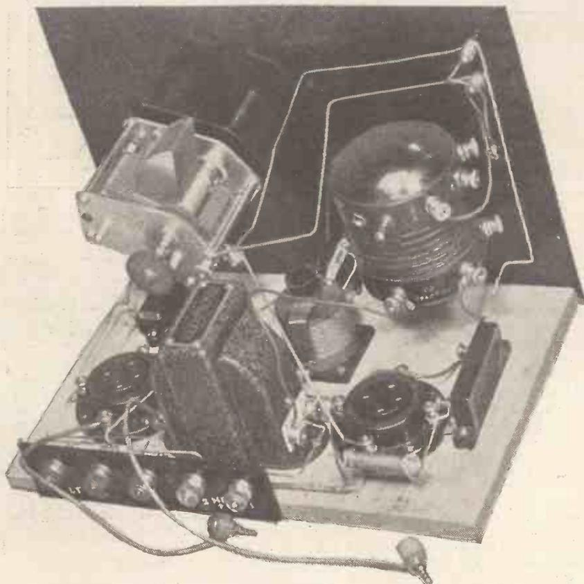
As the back of panel shows the grid leak is soldered directly into circuit. Two small clips could be used and there would be room to mount the component on the baseboard.
