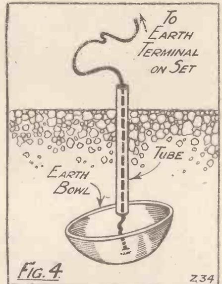
connections and that portion immediately below the run of the aerial wire. It is for this reason that the water-pipe earth sometimes gives poor results, the actual underground mains often being very remote from the position beneath the aerial.
