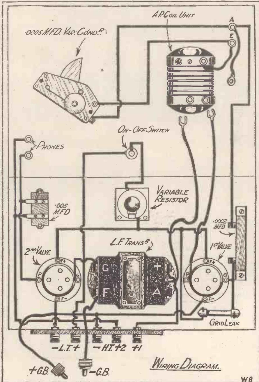
Note the lead connecting the Earth terminal to F-of first valve holder is not shown in this diagram.
