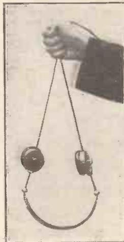
Fig. 7. One of the best methods of testing a pair of headphones.
