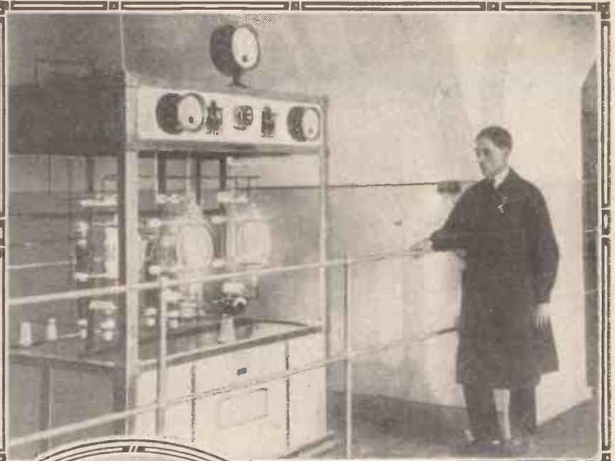
The photograph above shows the oscillator portion of the transmitter, which was constructed by Marconi's Wireless Telegraph Co.
