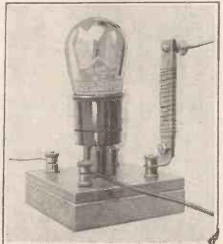
Fig. 4.—The resistor in place on the filament terminal of the valve holder.
