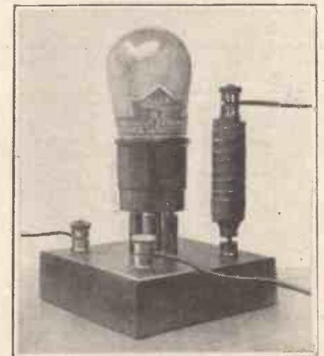
Fig. 10. A further type of resistance that is easily constructed.
