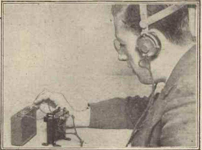
(Above.) If 'phones are connected across one winding of an L.F. transformer, and a battery is "tapped" across the other winding, corresponding loud clicks will be heard if the component is O.K.
