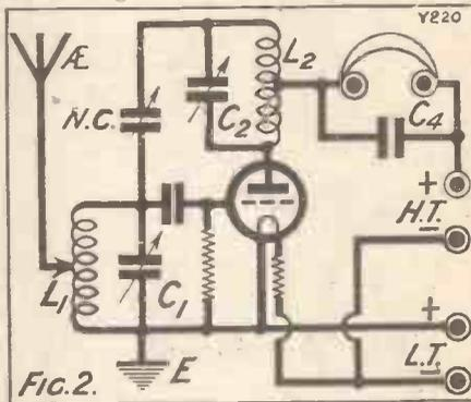
to  $C_1$ , the two condensers being gang controlled. The telephones were shunted by a fixed condenser  $C_3$  of the usual value of .0005 to .001.
