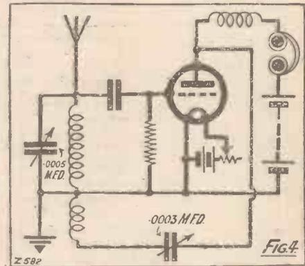
receivers, and these produce air waves and thus sounds can be heard. A certain amount of the energy in the plate circuit is fed back to the grid of the valve across the inductive linkage between the reaction coil and the aerial coil to be amplified again.
