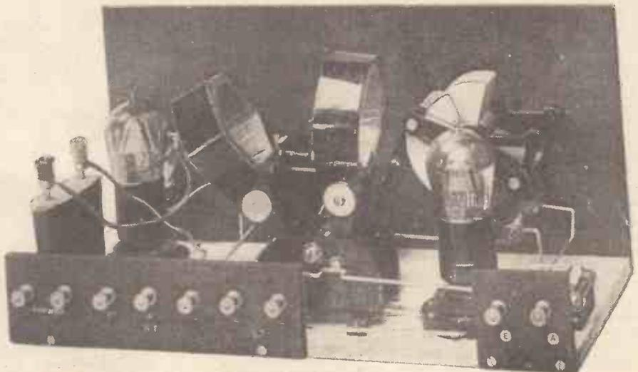
This receiver embodies the "swinging-coils" system of inductive reaction coupling.
