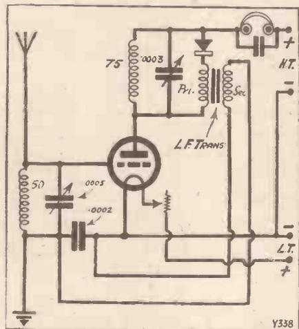
The correct connections for a one-valve reflex set, with parallel aerial tuning, are given above.
