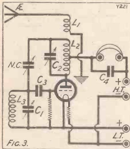
When this circuit was first tried out no shunting condenser was present across the telephones, for in view of the fact that they were connected to the nodal point of  $L_2$  I thought that a condenser of this description should not be necessary. I found, however, that it was impossible to get the set to oscillate satisfactorily unless this condenser was provided, and it was therefore put in as is usual in magnetic or tuned plate reaction circuits.
