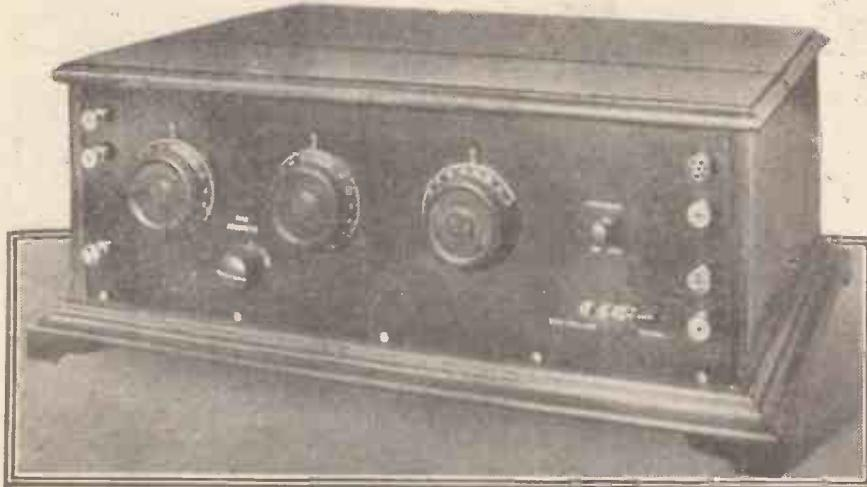
The three variable condensers (aerial, H.F. and reaction) have vernier dials, while a lossor control is provided for cutting down the volume when necessary.
