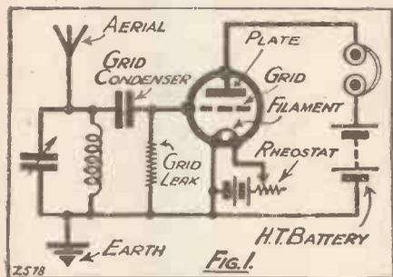
with other listener's reception. In effect, reaction can transform a wireless receiver into a transmitter and make it emit waves of its own which will mix up with the legitimate radio waves and thus upset radio reception in a whole district.
