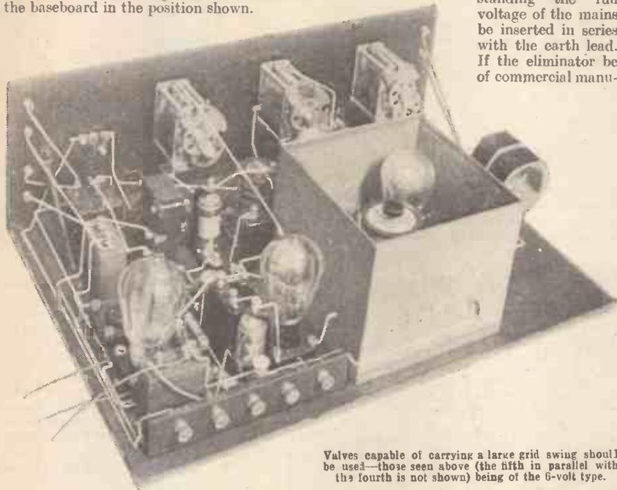
Valves capable of carrying a large grid swing should be used—those seen above (the fifth in parallel with the fourth is not shown) being of the 6-volt type.
