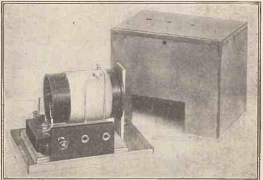
The complete wave-trap can be used with a metal screening box.
