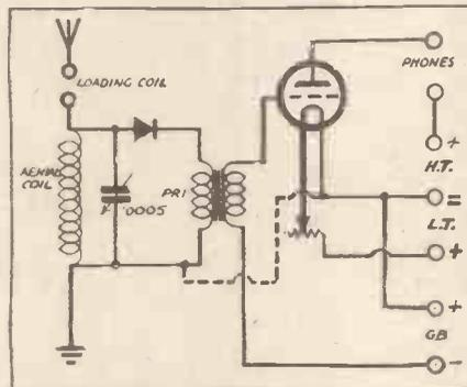
The above diagram is supposed to represent the connections of a crystal set and low-frequency amplifier, for receiving 5 X X or the local station; but it is wrong, and the set would not work properly.
