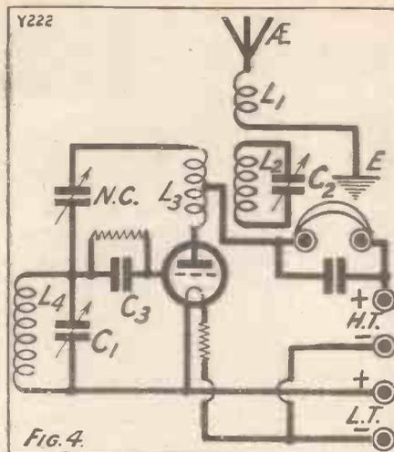
It was also found that using the neutralising condenser to bring the set on to the edge of oscillation very fierce reaction was obtained with a very large degree of backlash. It was therefore necessary to find another way of applying the principle which I had in mind for obtaining constant reaction.
