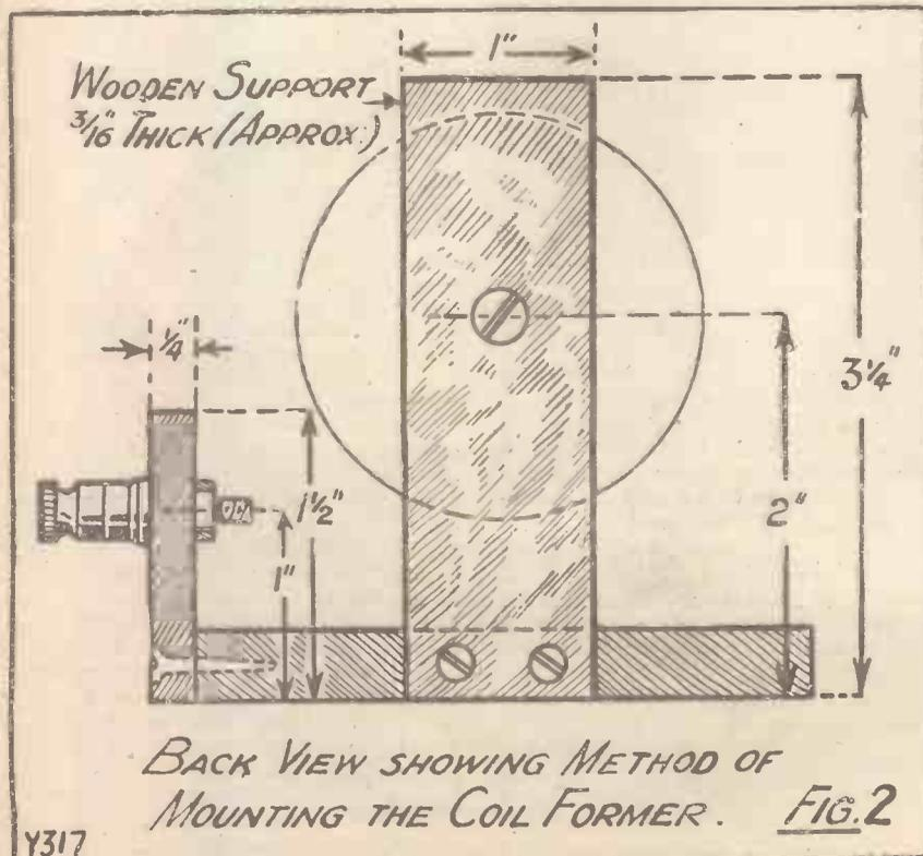
BACK VIEW SHOWING METHOD OF MOUNTING THE COIL FORMER. FIG. 2
