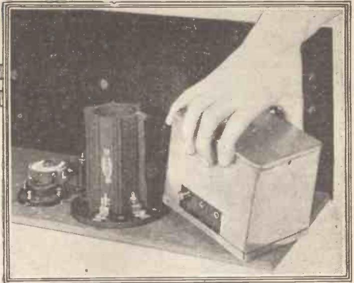
An efficient, easily-made and compact wave-trap which can be used in any type of receiver.
