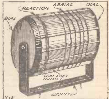
method adopted by the writer, which has the merit of being adaptable to different coil formers, is neat in appearance, perfectly rigid, and what is perhaps of equal importance, there is practically no constructional work.
