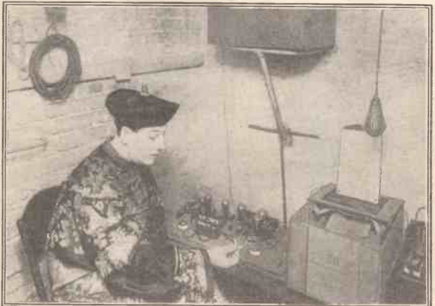
Switching on the amplifier and "mike" circuits. The "mike" is in the box on the right, comfortably packed to avoid extraneous pick-up.
