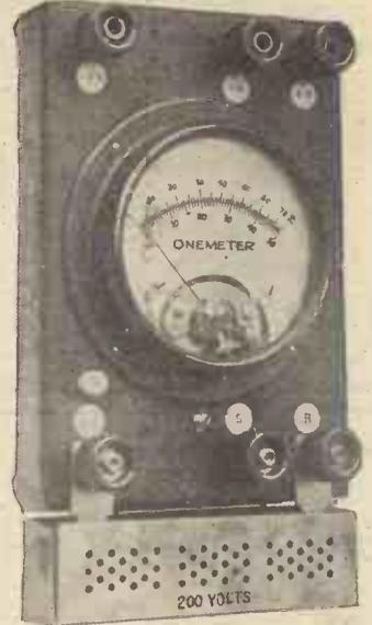
The ACONEMETER. Model VAC.3. In Case. Is a new Model measuring Alternating Current, a 3-range instrument reading 0-150 v., 0-300 v., and 0-600 v. Price, inclusive of case, 75/-, 1,500 volt Multipliers, 44/- extra. Get our New 72-Page Catalogue.
