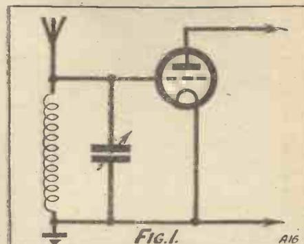
to plate, and to modify or alter its volume. (See Fig. 1.) When we connect up the H.T. battery, we make the filament of the valve negative and the plate of the valve positive.
