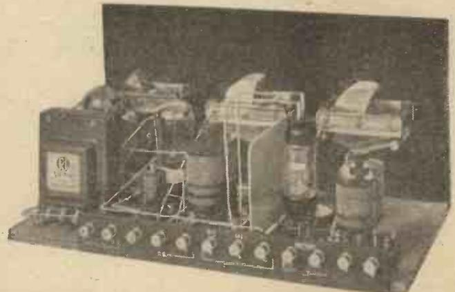
The peculiarity of the new screened-grid H.F. valve, one of which is shown in the above photo, is that it has a very high amplification factor, but its impedance is also of a high order.
