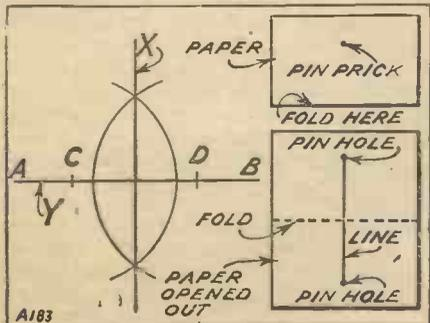
Temporary paper "squares" may quickly be made by folding a sheet of paper in half and placing a pin prick anywhere on the folded paper. Open the paper out and draw a line from one pin hole to the other. The result, when cut out, is a handy "square," formed by the line drawn and the line of fold made in the paper. Such a method may be used for cutting a permanent "set square" in celluloid or wood, the paper cut out being first used as a marking-out template. H. B.
