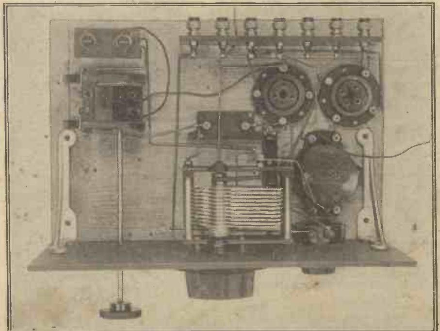
One of the features of the famous "Chitos" circuit is that it makes the optimum use of reaction effects. The moving-coil holder, which can be seen above, and a variable resistance, are the essential reaction controls.
