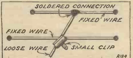
being made. The wire which is left disconnected at one end temporarily is secured to one of the fixed wires by means of a small clip, until the constructor is ready to fix the loose end. This simple little device will save a certain amount of time and work. H. B.
