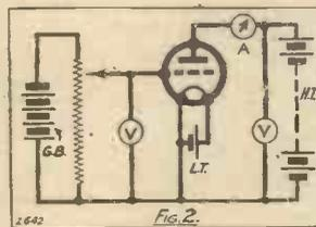
are the high tension and grid bias, but there is a third variable which is the filament potential of the valve itself. We can measure the amplification factor of the valve under all kinds of varying conditions, and we will find that there is but little change in its numerical value.
