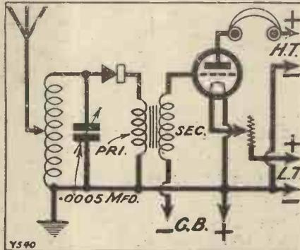
The correct connections for a Crystal and 1 L.F. receiver are shown above.
