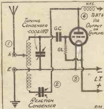
As explained in this article, the numbers show where spare components can be used to improve an ordinary one-valve reaction detector.
