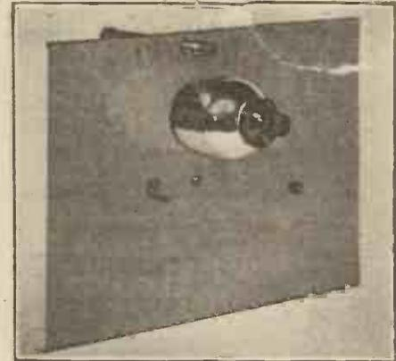
A valve holder and screen combination for use with screened-grid valves is one of the new lines exhibited by the Peto-Scott Co., Ltd.
