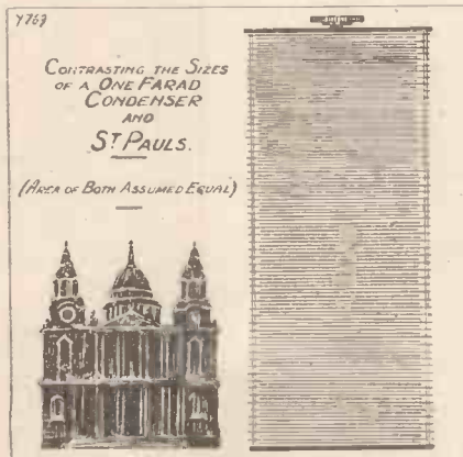
Contrasting the sizes of a 1-farad condenser and St. Paul's. The height of the condenser would be 790 feet.
