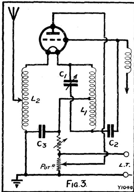
obtained without altering the capacity of  $C_2$ , control being quite as smooth as on normal wave-lengths. In tuning, very little hand-capacity variation was observed with an unscreened tuning condenser.
