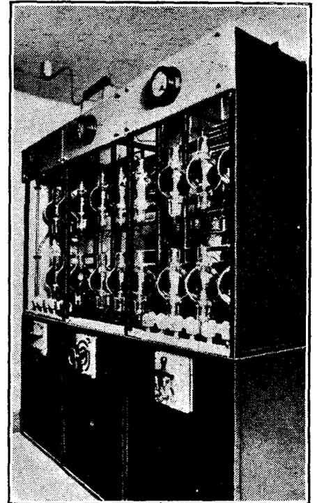
One of the huge rectifying panels. This portion of the Toulouse gear embodies 20 valves and rectifies the H.T. required for the transmitter.
