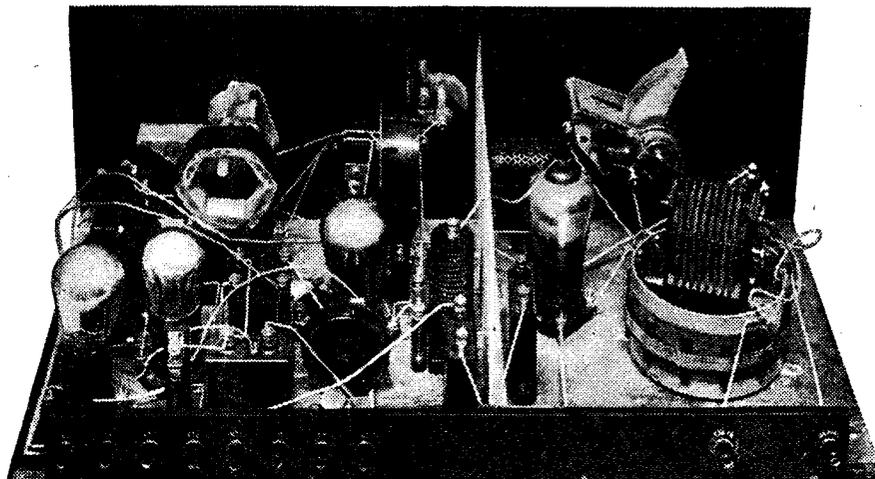
The flex lead to the top of the S.G. valve is an important one. Keep it direct and well clear of all others.
