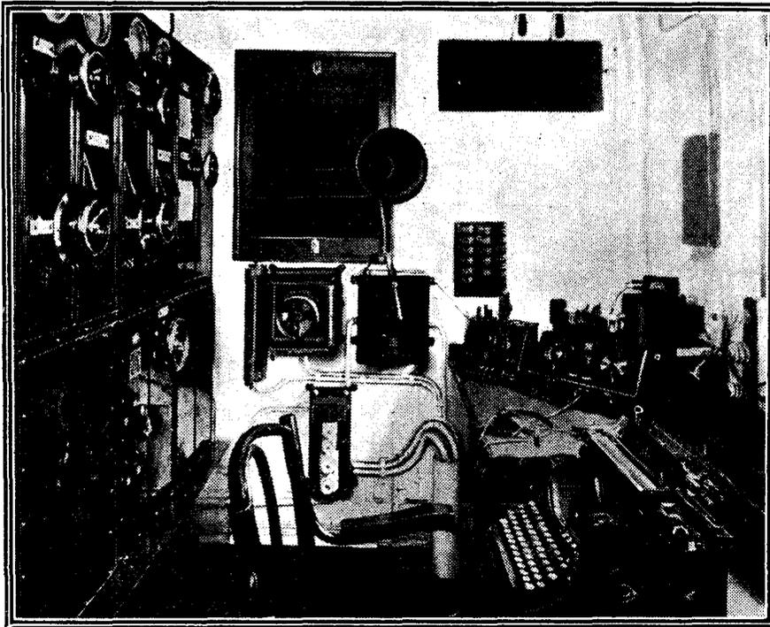
This is the 800-watt transmitter fitted on the ship "Ozeana." The receiving outfit can be seen on the right.
