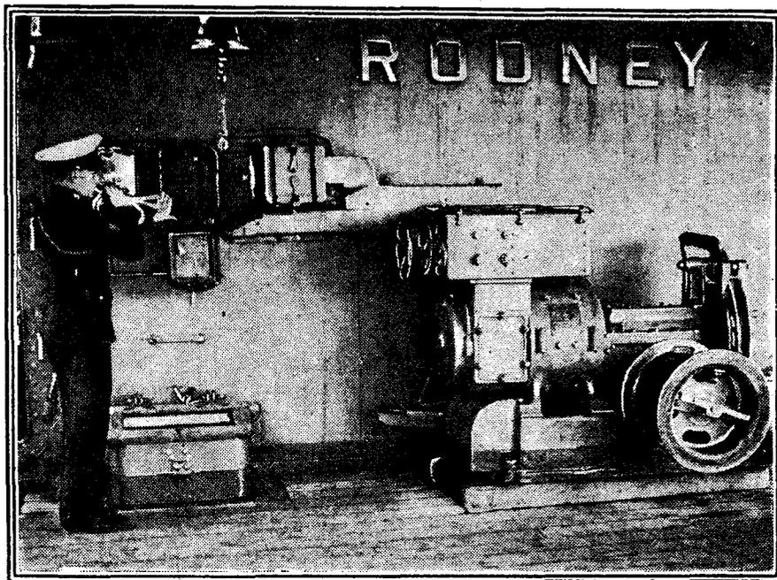
Three hundred loud speakers—the biggest collection on any ship in the world—are fitted on H.M.S. "Rodney," and here the bugler is shown sounding a call which is re-broadcast simultaneously in every part of the ship.
