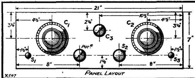
required, but by using one of the single-hole mounting type, we have avoided any awkward constructional work here. The two coils, you will notice, have been placed very carefully in the layout, so that interaction between the live and the dead one is prevented, and altogether we find this change-over scheme a very efficient one.
