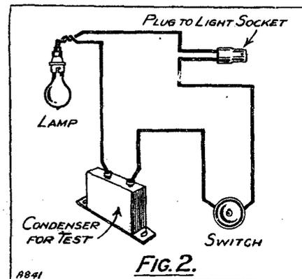
before attempting to touch the condenser, discharge it by "shorting" the two terminals together with a screwdriver.
