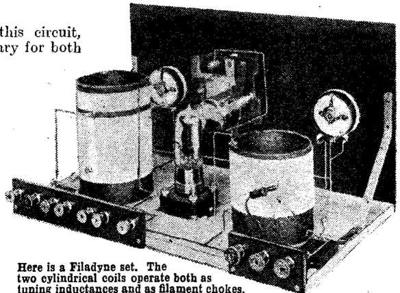
Here is a Filadyne set. The two cylindrical coils operate both as tuning inductances and as filament chokes.
