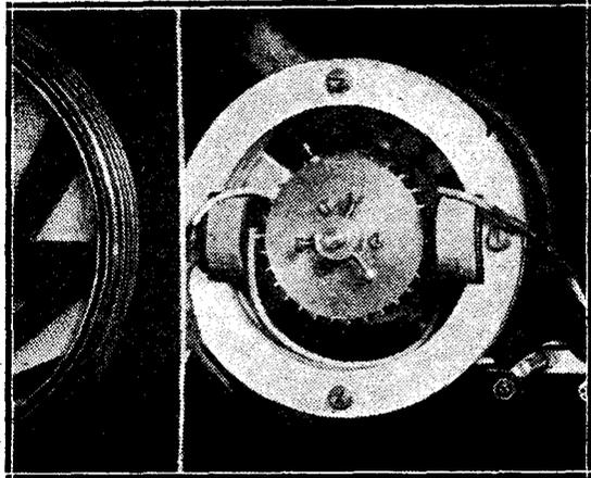
The automatic synchronising device used in the Baird Televisor.
