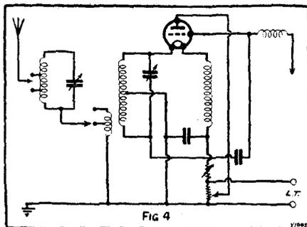
filament current under Filadyne conditions, so that there is ample margin on the rheostat to compensate for the extra resistance of the long-wave coils without increasing the voltage of the filament supply.
