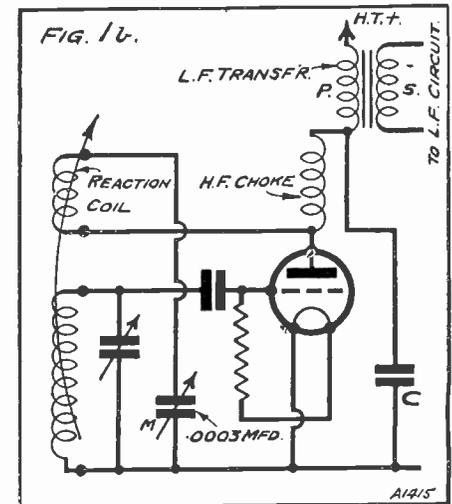
The circuit of Fig. 1a changed to capacity-controlled reaction.
