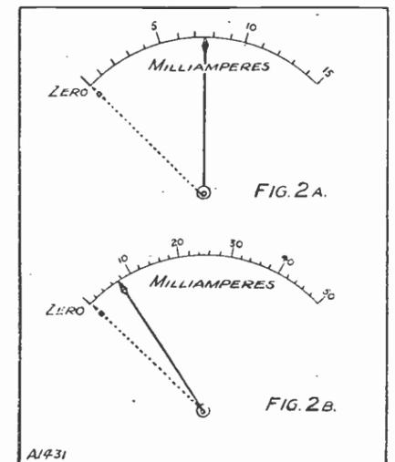
This drawing illustrates the importance of the relative sizes of the scales of meters. Notice the distances covered by each of the needles to indicate the same one or two milliampers.
