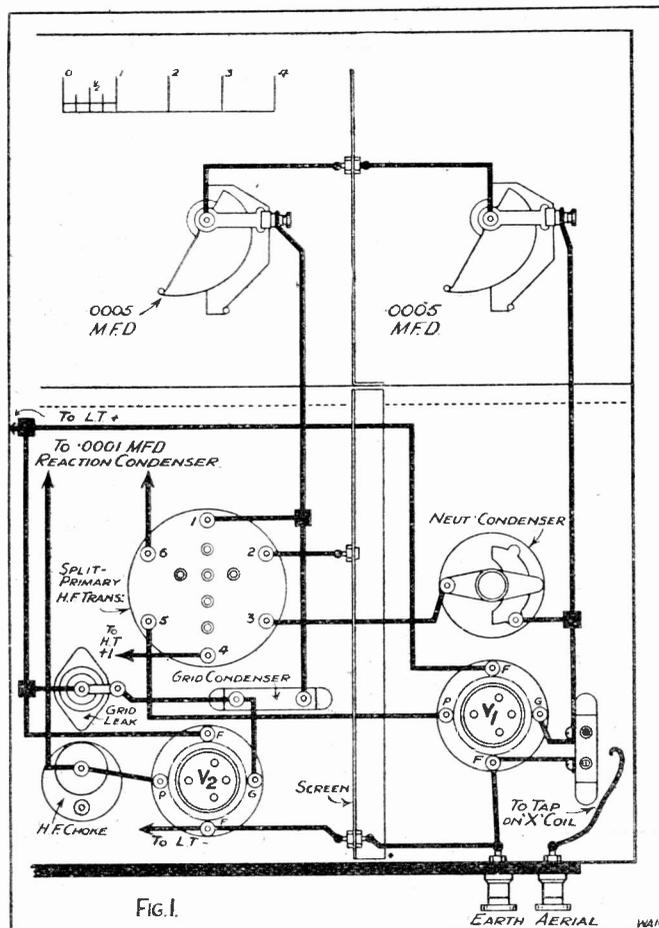
The H.F. side of a set employing a straightforward circuit, which can be modified quite easily to accommodate a screened-grid valve.
