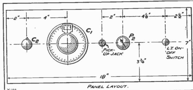
The panel is just like the "Magic" Three's, except for the pick-up jack and the volume control (P<sub>2</sub>).
