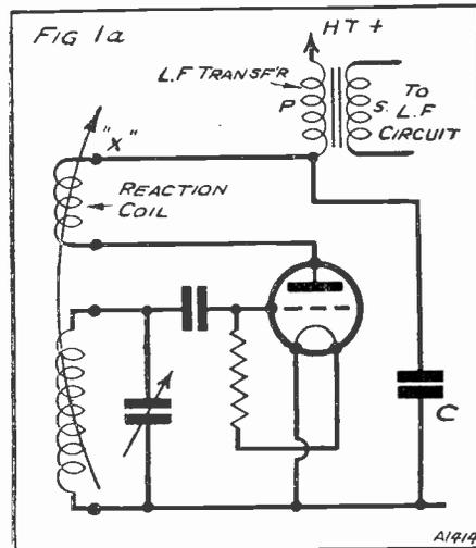
A typical circuit employing swinging-coil reaction.
