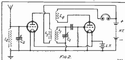
The new coil could be the coil of our original detector circuit, and the energy thus fed into it is exactly the original aerial energy amplified by the action of the wonderful thermionic valve.
