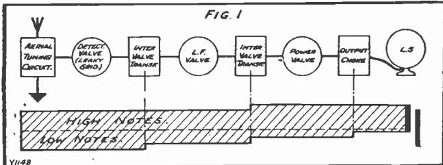
Here is shown an ordinary old-fashioned detector and 2 L.F. transformer-coupled set, which, as you see, has a rooted objection to low notes, and believes the piccolo is the only instrument worth hearing.
