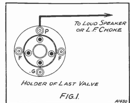
This is the wire you have to disconnect in order to insert the milliammeter when you use it to check the power valve's activities.
