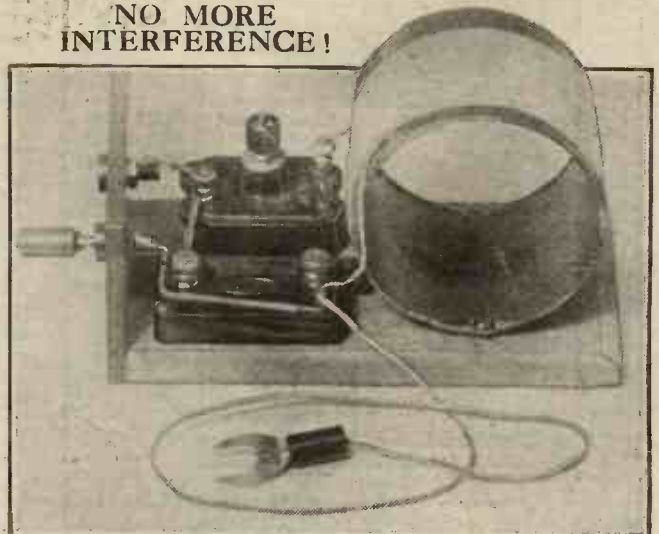
Here we see the complete rejector—a simple coil, a fixed condenser, a small pre-set variable, and there you are! Build it to-day and enjoy radio to the full.
