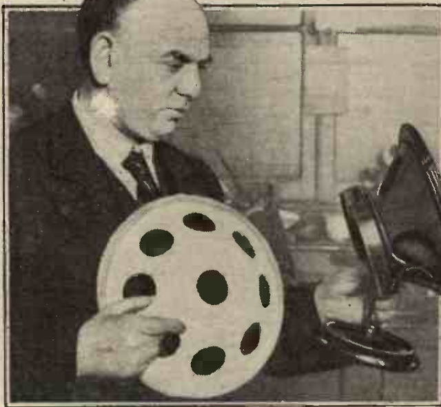
Mr. Samuels with two of his patent loud speakers (one is in an unfinished condition). They are made of compressed cotton, and Mr. Samuels applies the same principle of manufacture to the production of synthetic wood.
