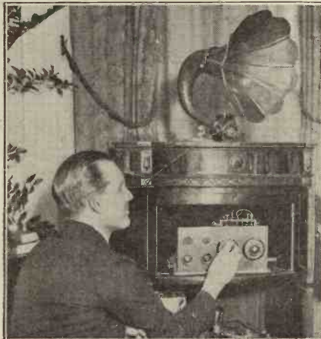
The position of the loud speaker and of its leads may have a marked effect upon results, and very often a howl can be cured by moving the loud speaker.
