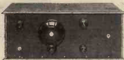
The operating controls are really only the large dial in the centre (tuning), the one to the right above (reaction) and to the right below (volume). Those to the left control the rejector, and only require occasional manipulation. Remember that the rejector setting is sharp and calls for care.
