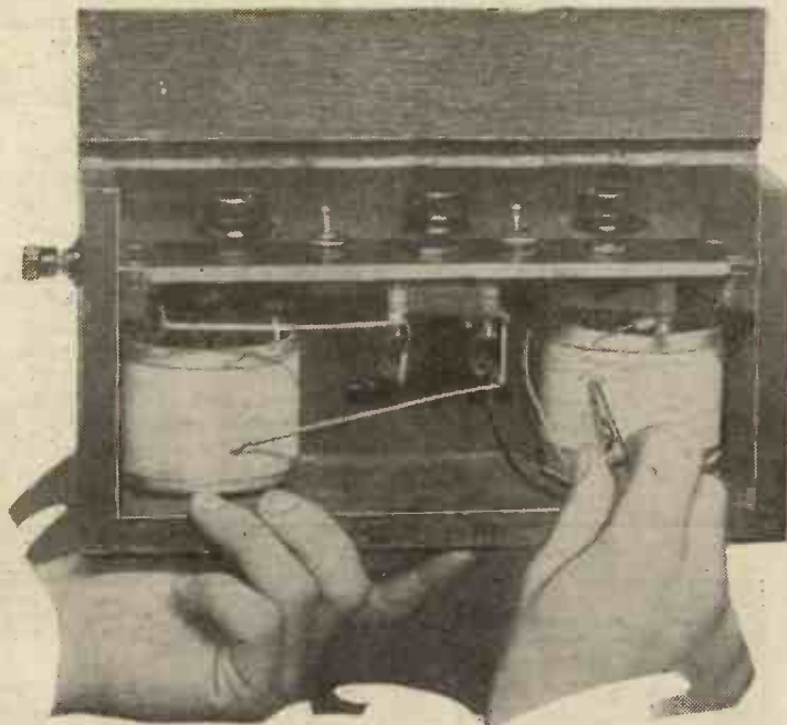
The coil on the right has a number ofappings to one of which a clip is taken, as shown. This adjustment has only to be made in the first instance when "setting" the Rejector, after which you flick the switch on, and out goes the unwanted programme!
