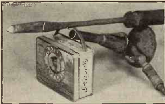
One of the best ways to heat a soldering-iron is to use a bunsen burner. A stand can be improvised quite easily, the rest for the iron being a piece of brass or copper strip fixed to a tin box. We don't say it's elegant, but we do say, from experience, that it simplifies soldering by heating the iron quickly and cleanly.
