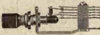
Jack Switch. Of entirely new design, brass frame, heavily nickel-plated, springs of nickel silver, the contacts being riveted in. The control contact is of the push-pull type. Prices from 2/9 to 4/6
