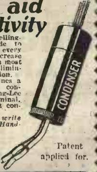
Connect the new Belling-Lee Condenser Spade to your aerial lead. In every case it will greatly increase the selectivity, and in most cases it will entirely eliminate the unwanted station. This new idea combines a .0002 series Aerial condenser with a Belling-Lee clip-on Spade Terminal, which ensures perfect contact.
