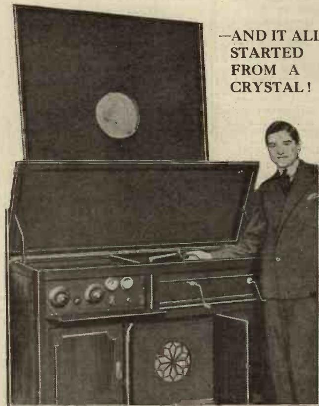
Six years ago, when at school, he made a crystal set, and then he got "valve fever" and made bigger and bigger sets, giving more and more volume. This outfit is a seven-valve Radiogram receiver, with two double-spring motors, and two 12-inch turntables. The volume of sound is said to be "equal to three bands"—and yet it was a spare-time job!
