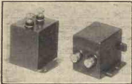
Two examples of large-capacity "paper" condensers from the comprehensive T.C.C. range.
