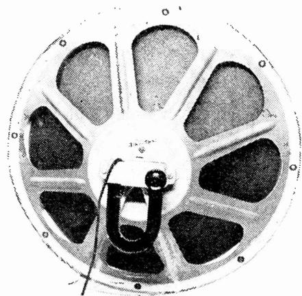
Here is the famous "Blue Spot" L.S. Unit mounted on its chassis and ready for placing inside your own cabinet.
