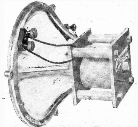
The ends of the leads going to the moving coil are clearly shown in this Goodman M.C. Speaker.
