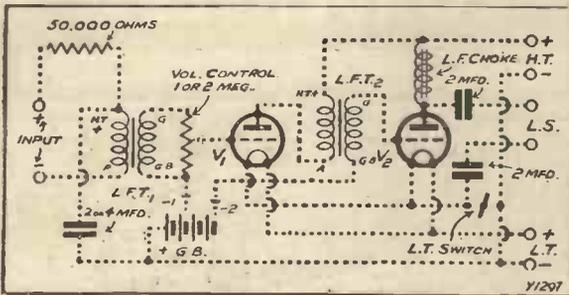
Here are the connections of last week's two-valve amplifier, shown by the dotted lines. It can be used with a crystal or small valve set and will give great power and purity, with the advantages of volume control and choke-filtered output.
