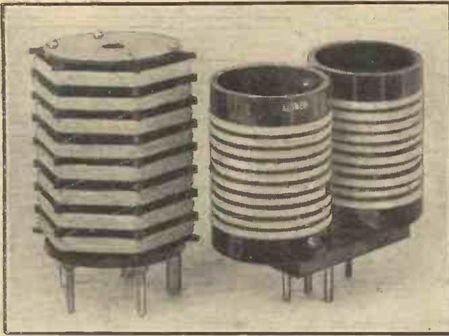
A pair of special Listen coils of the interchangeable type with sectionalised windings for long-wave work.
