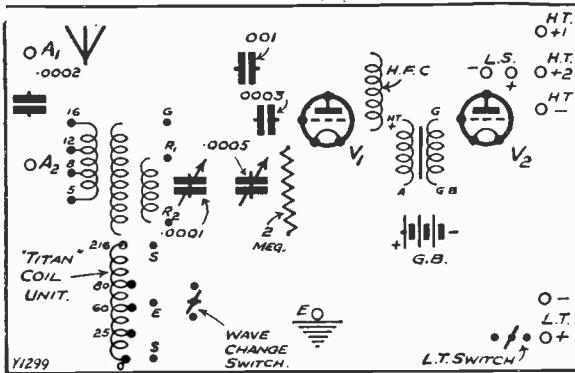
Here are all the necessary "components" for a two-valve set (Det. and L.F.) with a "Titan" tuner for wave-change. The .0001 reaction condenser has a .001 fixed condenser in series with it, to prevent shorting, and the circuit is otherwise perfectly straightforward. Could you wire it up? (Look out for the answering diagram next week.)
