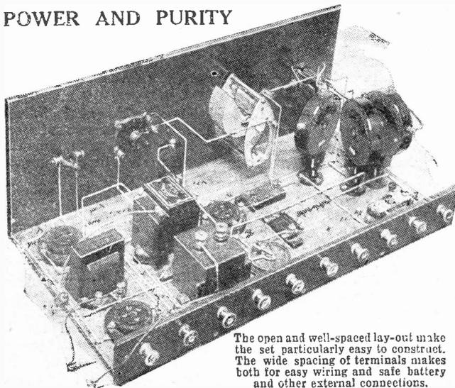
The open and well-spaced lay-out make the set particularly easy to construct. The wide spacing of terminals makes both for easy wiring and safe battery and other external connections.
