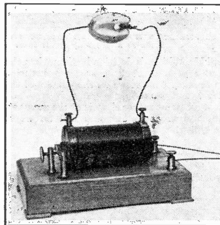
A small induction coil can be used to provide a fairly good indication of the efficiency of an insulator.
