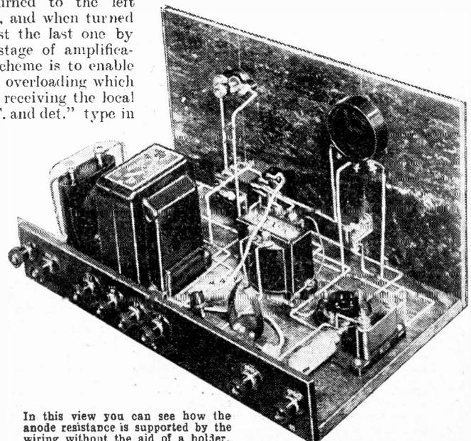
In this view you can see how the anode resistance is supported by the wiring without the aid of a holder.
