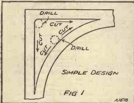
Saw cuts should always be made towards sharp corners, as even a fretsaw will give a rounded effect which looks "amateurish."
