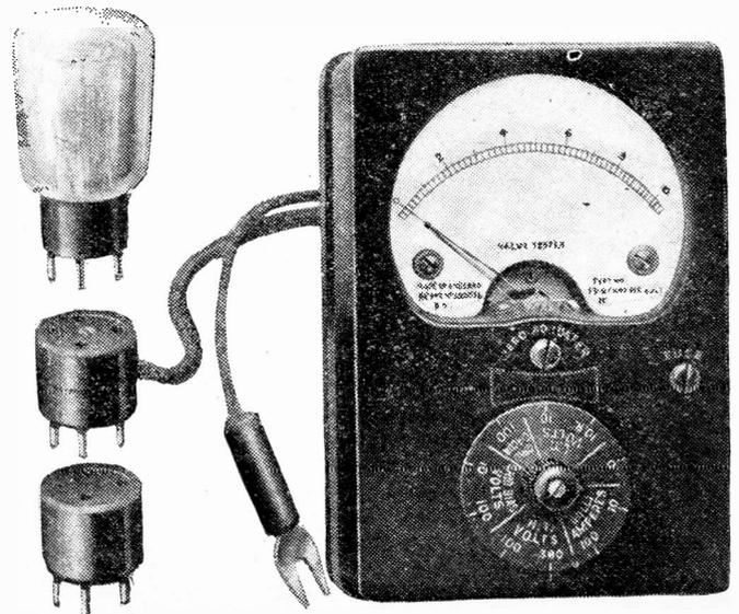
Showing how the Ferranti Valve Tester plug takes its place between a valve and its ordinary holder.
