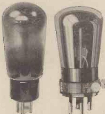
The valve on the left is a Vatea rectifier made by Abbey Radio, and the one on the right a Dario rectifier.
