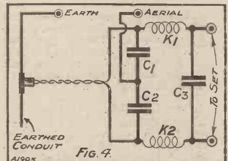
This shows the connections for using the house wiring to pick up broadcast energy.
