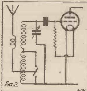
A simple wave-change added to the Fig. 1 circuit.
