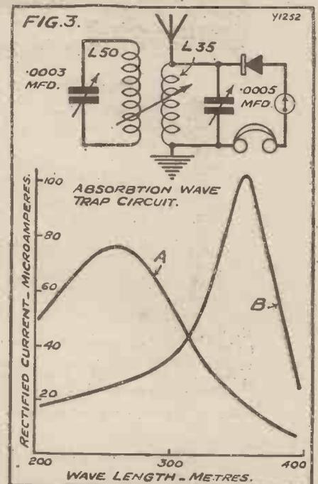
In the above three illustrations you see the various circuits tested, together with curves showing the results obtained.
