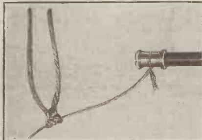
An aerial lead-in that swings against a gutter, or walls of a house, may give rise to scratching noises in your reception. It can be prevented, of course, by tying the lead-in away from the wall as shown above.
