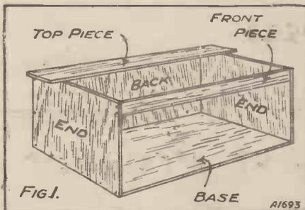
FIG. 1. This is a typical cabinet frame roughly knocked up.
