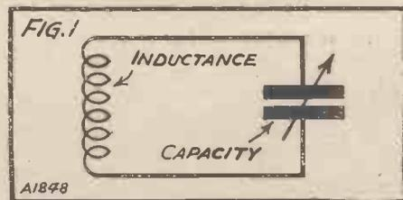
This is a diagrammatic representation of the simplest possible oscillatory circuit.
