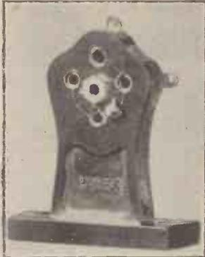
One of the most interesting components on show—a "Parex" screened-grid valve holder (Paroussi).
