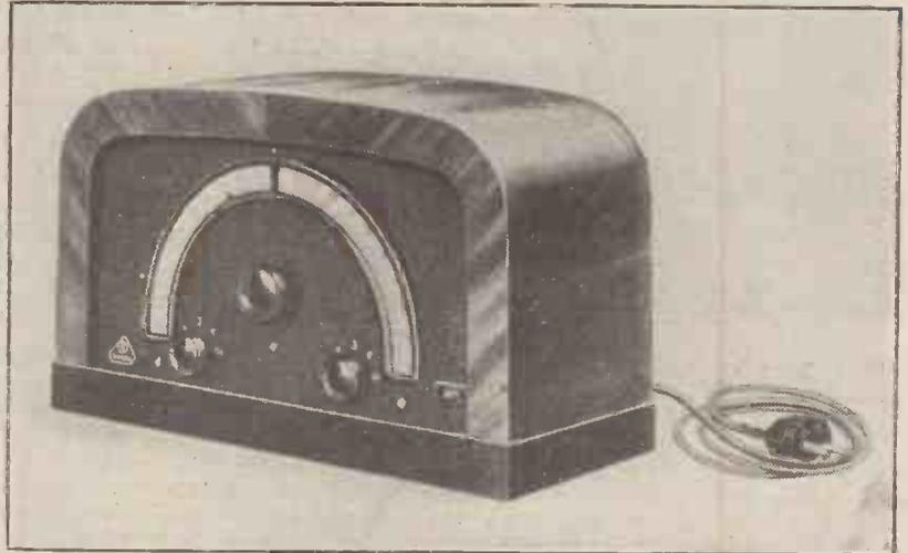
The most interesting thing about this all electric two-valver is the huge tuning scale extending over most of the front panel. Tuning is carried out by means of the knob in the centre, and extremely fine variation is possible.
