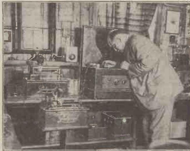
A German experimenter operating a machine that transfers radio programme items on to metal records, which can be used on any ordinary gramophone. The results compare very well with those given by the well-known wax recorders that can be seen in the photo.
