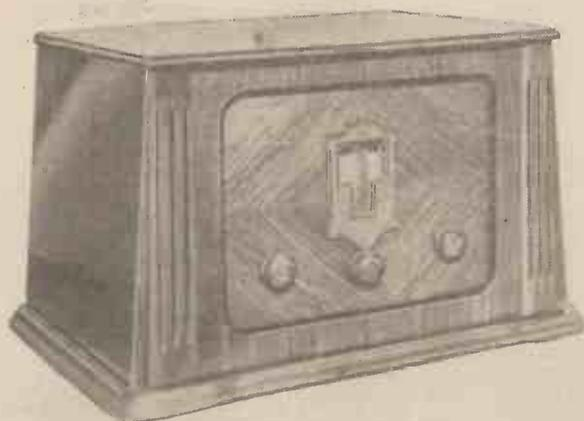
This is a Varley all-from-the-mains receiver, counteracted, so that a set running from the mains can be absolutely silent just like the set running from batteries.
