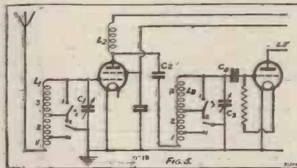
Mr. Allinson's new scheme applied to a circuit embodying an H.F. stage.
