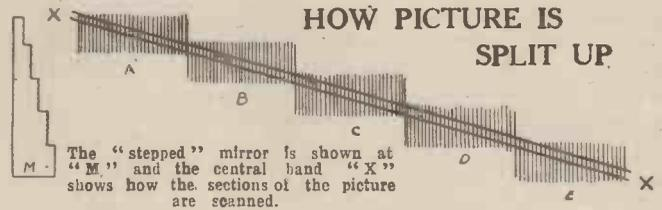
The "stepped" mirror is shown at "M" and the central band "X" shows how the sections of the picture are scanned.
