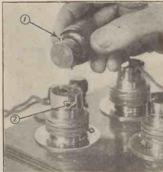
This view illustrates a simple method of ensuring that the adapter plug on the end of the twin flex lead from the accumulator always goes into its alternative sockets the right way round. Use an adapter of the wooden variety, and insert a small round-head screw exactly as you see at (1) above. Then file away a little of the metal of the holders as at (2) to admit the screw shank at one side only.
