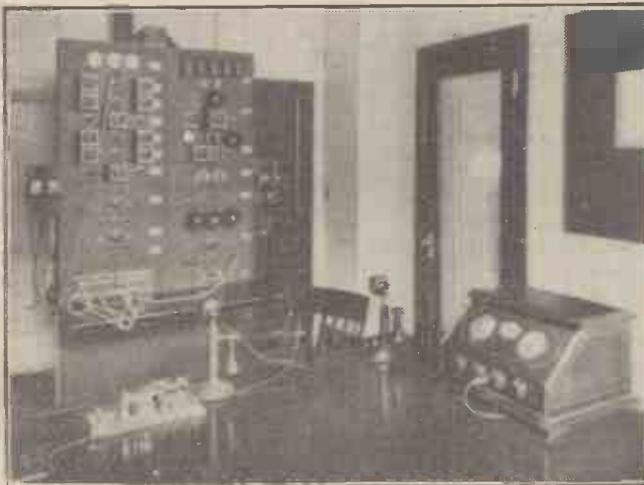
The control board linking the C K G W studios at Toronto with the transmitting station forty miles distant.
