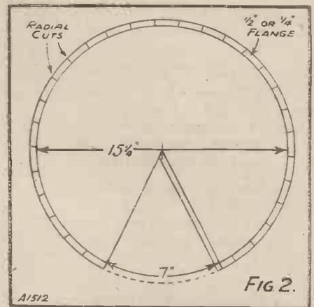
How the paper is cut to enable it to be bent into shape.
