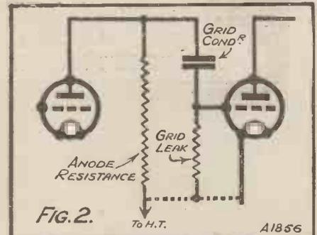
There must be a definite relation between the values of the grid condenser and grid leak if you want best results.
