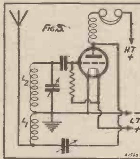
Here the extra aerial coil is eliminated, the reaction winding being made to do two jobs.
