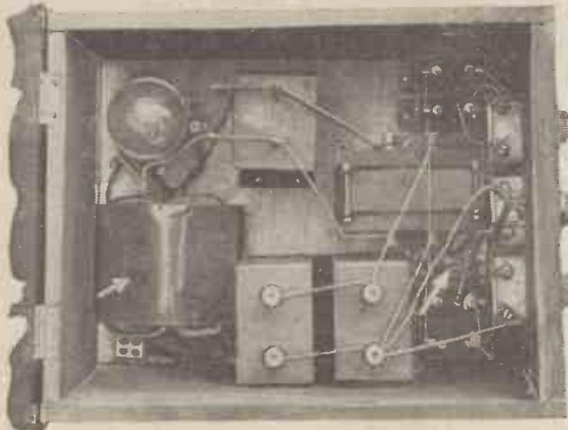
The mains unit in which a mouse built a nest. The arrow to the right indicates the shreds of paper carried in to form the nest, while the left-hand arrow points to the transformer, on the prints can be discerned.
