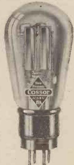
A full-wave rectifier made by Cosson.
