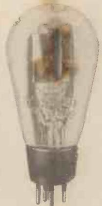
A full-wave Osram rectifying valve above, and below is one of the house dry rectifiers. Right, a well mains transformer.
