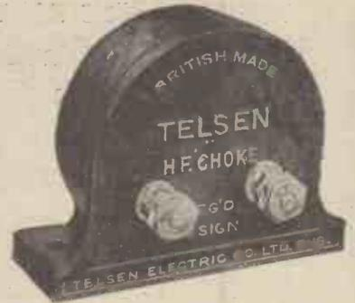
Telsen H.F. Chokes, designed to cover the whole wave-band range from 18 to 4,000 metres; extremely low self-capacity. Inductance—150,000 microhenries. Resistance—400 ohms.
