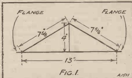
Here are the dimensions of a useful size of cone.
