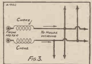
Air-cored chokes can be used to stop H.F.
