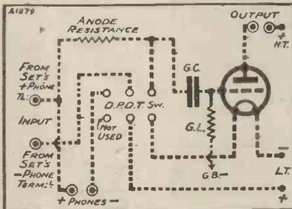
The dotted lines above indicate the connections for the amplifier, the components of which were given in last week's "Wirelet."
