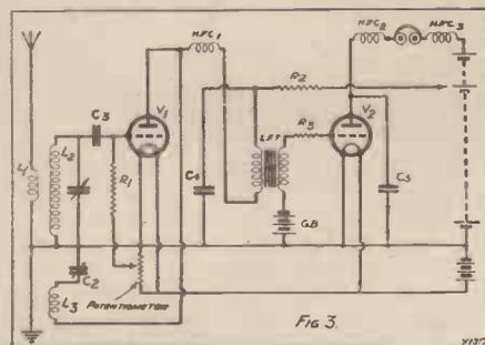
H.F. chokes and resistances used to confine the H.F. to its own parts of the circuit.
