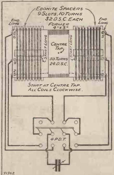
wound as a continuation and finished at tag No. 2. This completes the short-wave coil.
