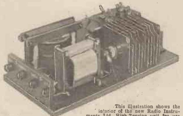
This illustration shows the interior of the new Radio Instruments, Ltd., High Tension unit for use with A.C. mains. The protective covering has been removed, and it will be seen that a metal rectifier is embodied in this instrument.
