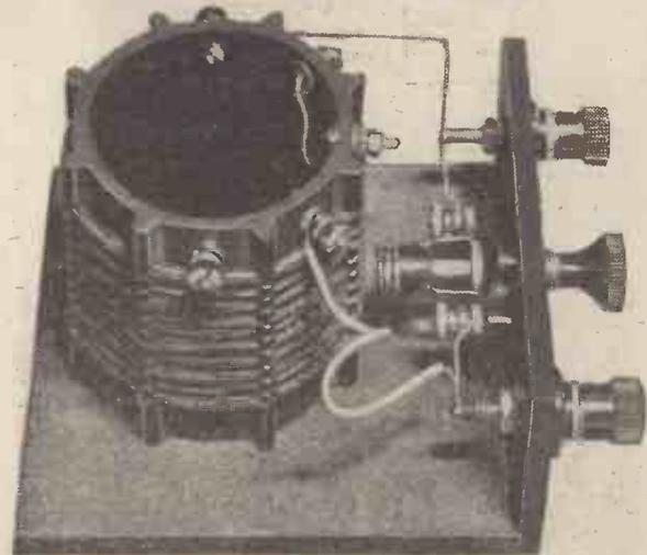
You can do so easily if you build the "Contradyne." No longer need you suffer that "butting-in" of the low-wave local on your long-wave programmes. Just try the flex lead on the various terminals on the coil, and you will soon find the right adjustment for your conditions.
