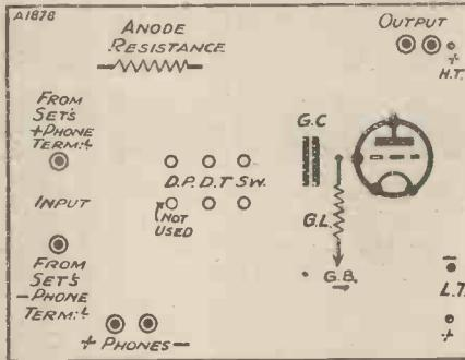
The "components" shown above are those necessary for a one-valve amplifier (resistance coupling) with a switch to listen on 'phones to the set itself, when desired. The idea is that the amplifier is joined up to the set and then the D.P.D.T. switch gives you either "set only" or "set with amplifier" without the necessity of changing connections. Can you "wire up" the circuit to bring in the extra valve by means of the switch shown?
