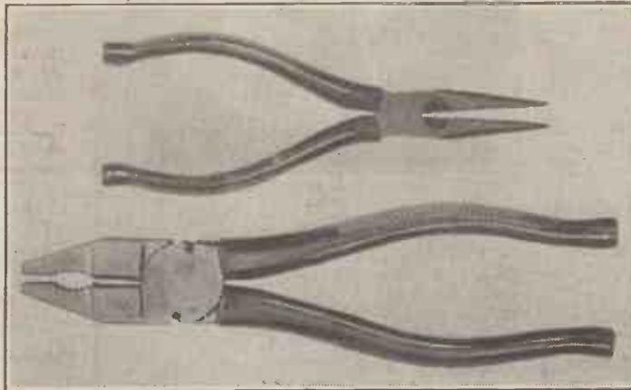
Ever tried insulated pliers? If you have to work with "live" wires sometimes they are very useful, saving the worker from shock and preventing shorts. Different kinds can be obtained, two very useful models being shown above.
