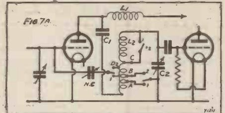
Shunt feed stops the H.T. from flowing through the coil.
