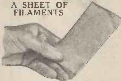
Tungsten, which is extensively used for valve filaments is seldom seen in sheet form. There is enough metal in this piece for many thousands of filaments.
