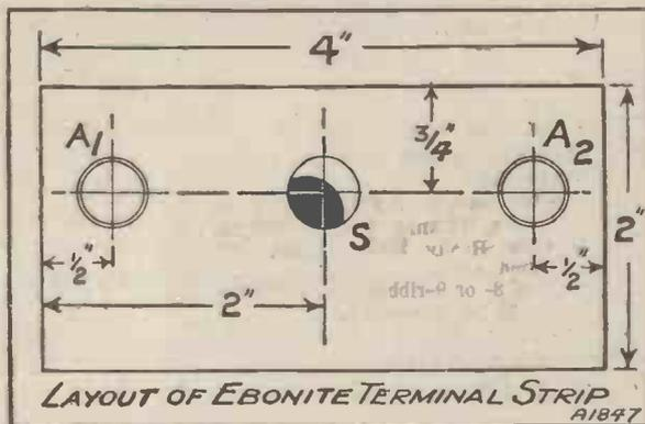
Just connect your aerial to A<sub>1</sub> and wire A<sub>2</sub> to the aerial terminal on your receiver. For work on the lower wave-band close switch S, so cutting the "Contradyne" out of circuit. Pretty easy, isn't it?
