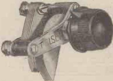
Telsen Variable Condensers (Bakelite Dielectric). Particularly designed for use as a reaction condenser, may also be used as a neutralising condenser where large capacity is necessary. All vanes are insulated with Bakelite which eliminates the possibility of a short-circuit between the moving and fixed vanes. Made in three capacities: '0005, '0003, '00015, supplied complete with pointer knob with one-hole fixing for panel mounting. Price 3/- each
