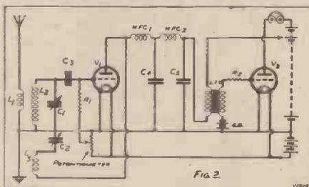
Adding a potentiometer enables the grid potential to be adjusted closely.
