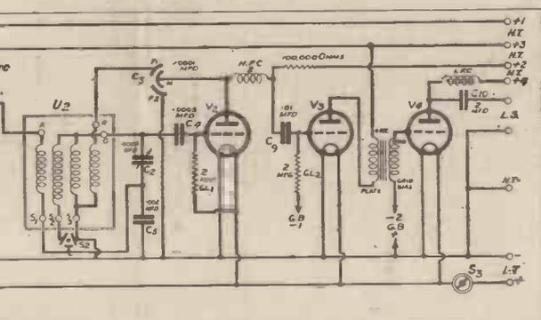
of the different circuits you see here, you will soon begin to realise what can be done by this first set of "P.W.'s" new series. Note the special methods of wave-change switching and the very simple wave-change switching.
