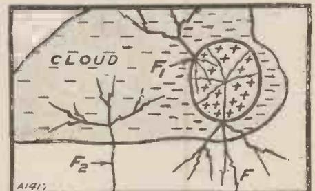
Fig. 2. The actual lightning discharge commences inside the cloud itself.
