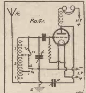
One coil only is used for long and short waves tuning, as well as for aerial coupling and reaction!
