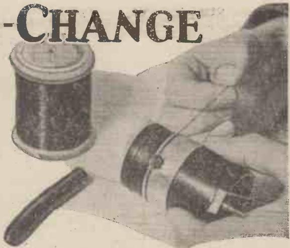
ONE of the complications in designing a wireless receiver for use in England is the fact that it has to be designed to cover two wave-bands. Ours is not the simple problem of meeting the requirements of a single wave-band from 200 to 600 metres, for we have also to cater for the 1,000 to 2,000-metre band.
