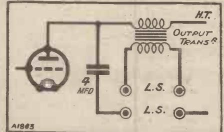
Mr. Mee used one winding of the L.F. transformer as a choke, and connected a second speaker to the other winding.
