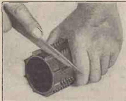
There is no doubt about the success of this little unit, the coil-former of which is slotted, as shown above. It is 2½ in. in diameter over the ribs and about 3 in. long. There are 10 file cuts in each rib, making 10 slots for the windings. The slots are about ¼ in. wide, and there is about 1-16th in. between them. Wind 20 turns of No. 26 D.S.C. in each (200 in all), tapped as in circuit diagram. Take ends and taps to small terminals mounted in former (see photos and wiring diagram).
