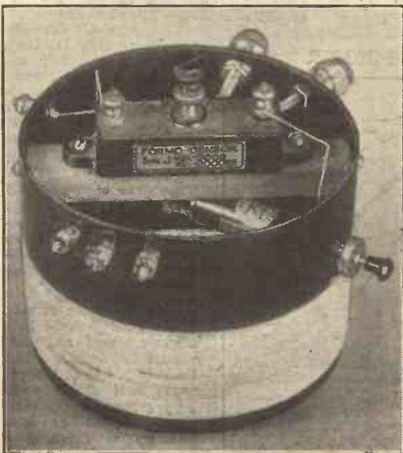
The only adjustments necessary are those of the little compression condenser and the crystal detector, and yet the set is wonderfully effective.
