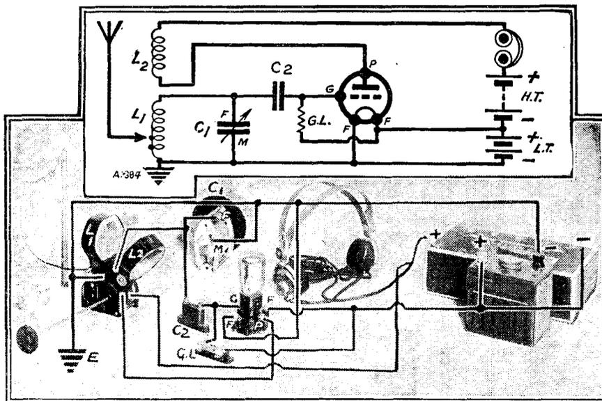
Here is a complete one-valve circuit with "swinging-coil" reaction. The components in the photo are connected up exactly in accordance with the theoretical circuit above, and all the lettering appears in its correct order. See if you can identify all the components and follow out their connections.
