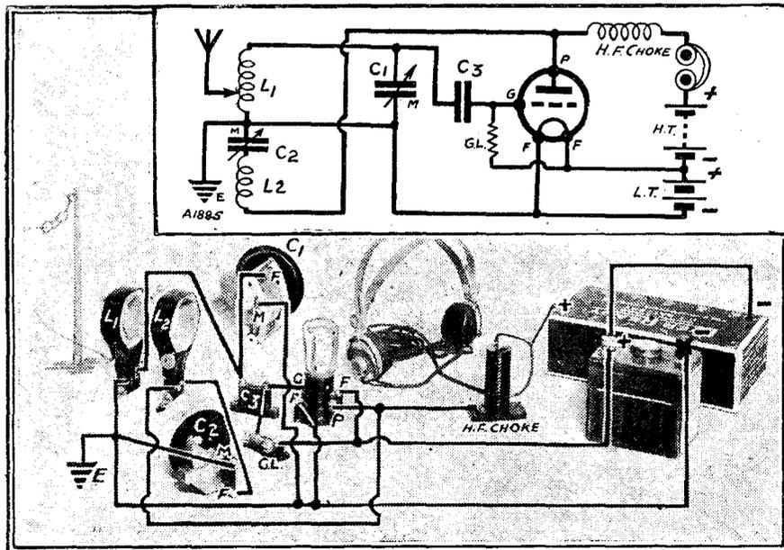
This circuit embodies a rather more complicated reaction system, but you should have little difficulty in tracing it out with the aid of "Pentode's" specially prepared picture.
