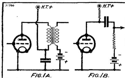
Whereas plain transformer coupling is likely to provide threshold howl, resistance coupling is almost immune from that fault.
