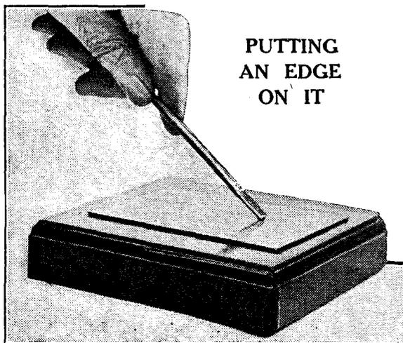
Trimming a screwdriver's edge on the home-made oilstone.
