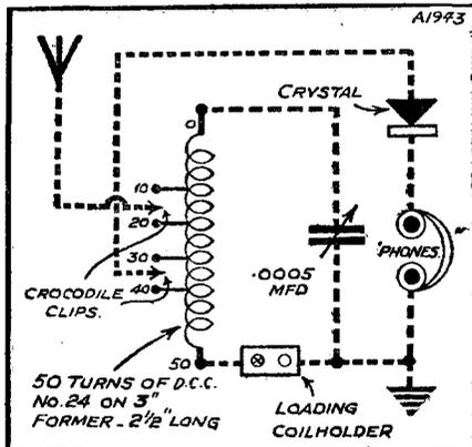
The connections for a good crystal circuit (based on a home-made coil and the other "components" shown last week) are indicated by the dotted lines above.
