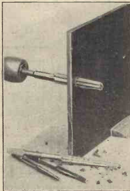
The reamer is often looked on as an extravagance, and many constructors enlarge a panel-hole by penknife and patience. But in its own limited field the reamer is invaluable and makes panel-drilling a pleasure.
