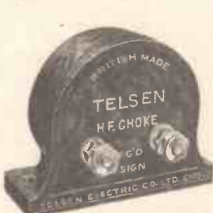
TELSEN H.F. CHOKES. Designed to cover the whole wave-band range from 18 to 4,000 metres, extremely low self-capacity, shrouded in genuine Bakelite. Inductance 150,000 microhenries. Resistance 400 ohms. Price 2/6 each.
