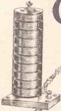
The H.F. choke (above) is a Wearite, for heavy-duty mains work.
