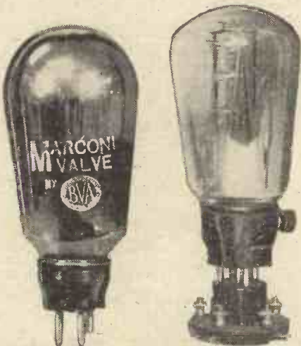
The P.X.4 and the Mazda A.C. Pen, two valves designed for output work. The former takes about 50 m/a. (max) and the latter 25-30 m/a.
