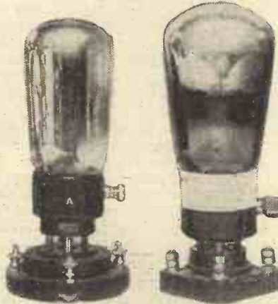
Pentode valves are inclined to "walk-off" with more milliamps than we expect. The Lissen on the left is fairly economical, while the 2-volt Mullard takes a total of about 16 m/a. max.
